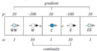
$$\int_{V_W} \frac{\partial u}{\partial x} dV = (u_C - u_{WW}) \frac{V_W}{2\Delta x_W} = (1 - 1) \frac{V_W}{2\Delta x_W} = 0$$
