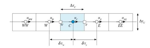
$$\underbrace{\dot{m}_{e}u_{e} + \dot{m}_{w}u_{w}}_{Convection} - \underbrace{\left[\left(\mu \frac{\partial u}{\partial x} \Delta y\right)_{e} - \left(\mu \frac{\partial u}{\partial x} \Delta y\right)_{w}\right]}_{Diffusion} = - \int_{V_{C}} \frac{\partial p}{\partial x} dV$$
