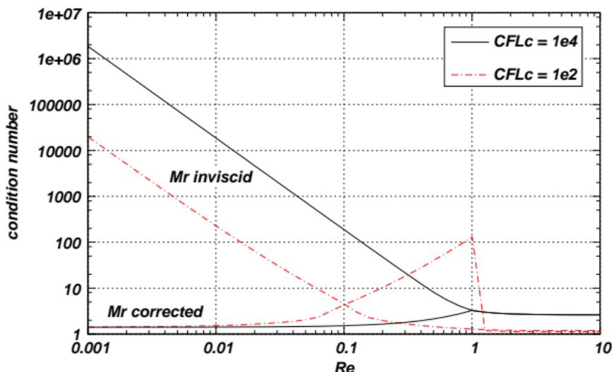
Condition number as a function of  $CFL_c$  for several Reynolds numbers with the reference Mach for the inviscid case ( $M = 1 \times 10^{-3}$ ).
