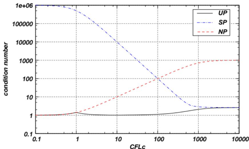
Condition number as a function of  $CFL_c$  with  $M = 1 \times 10^{-3}$  and  $M_\epsilon = 1 \times 10^{-6}$  for the inviscid case.
