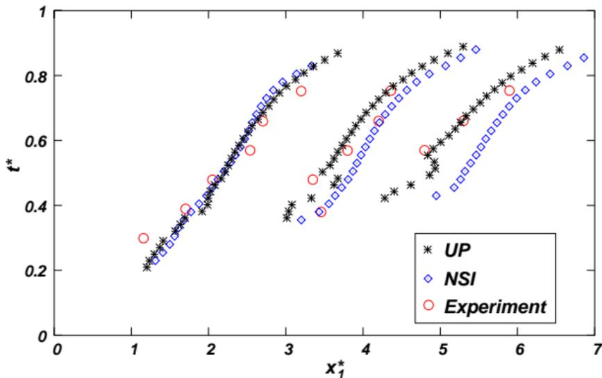
Comparison of predicted and experimentally observed positions of the first three vortices center.
