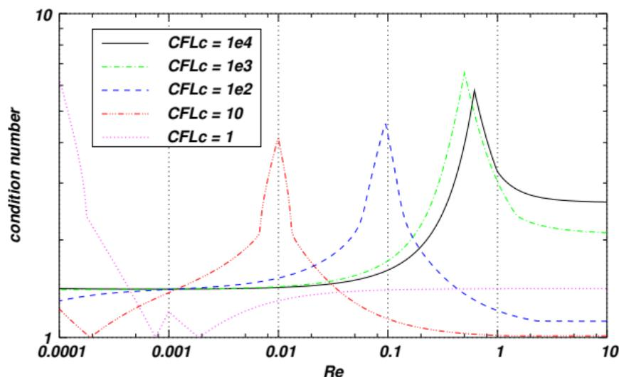
Condition number as a function of the Reynolds number for several  $CFL_c$  numbers for the viscous case.  $M = 1 \times 10^{-3}$  and  $M_\epsilon = 1 \times 10^{-6}$ .
