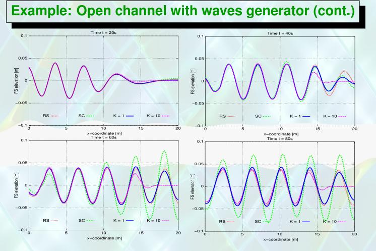
Free surface elevation for the reference solution (RS), the solution in the short domain with slip condition at the outlet (SC), and the last two solved with absorbing boundary conditions (ABC).
