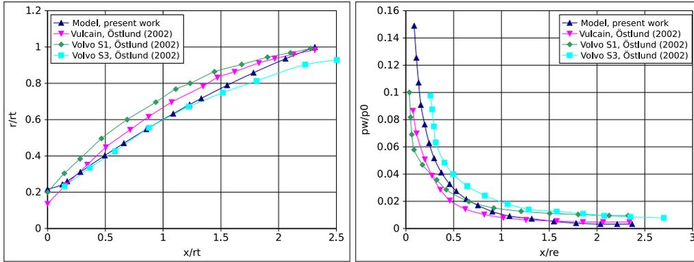
Figure 8: Radius and wall pressure distribution.
