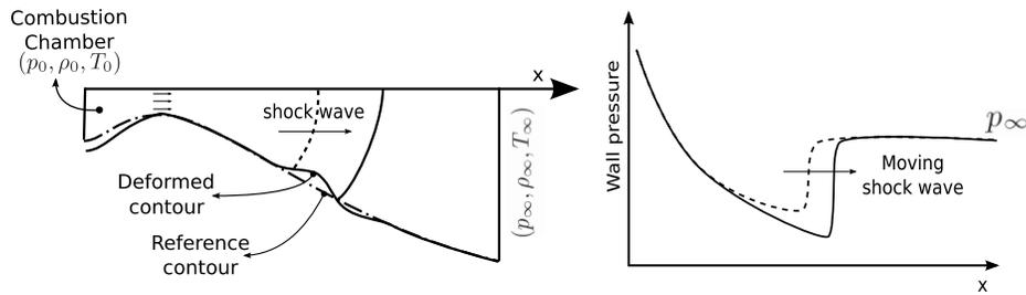
Figure 9: Schematic deformation of the structure.
