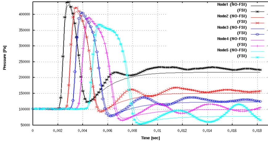
Figure 11: Wall pressures during the start-up. Comparison between NO-FSI and FSI cases.
