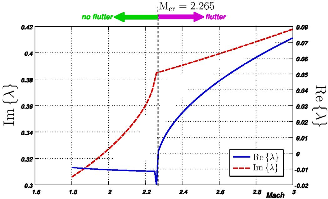
Figure 3: Lowest frequency mode for test case. Galerkin/Houbolt model.
