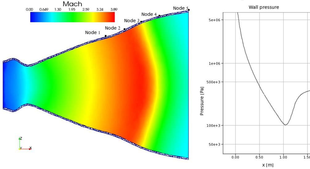
Figure 10: Structure deformation and pressure distribution for the moving shock wave.
