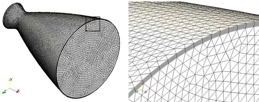
Figure 7: Spatial discretization for the fluid and for the structure.
