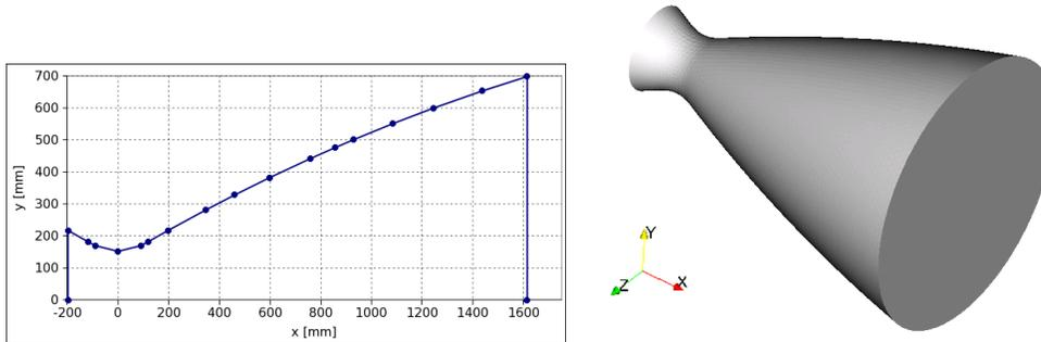
Figure 6: Contour line and 3D model.
