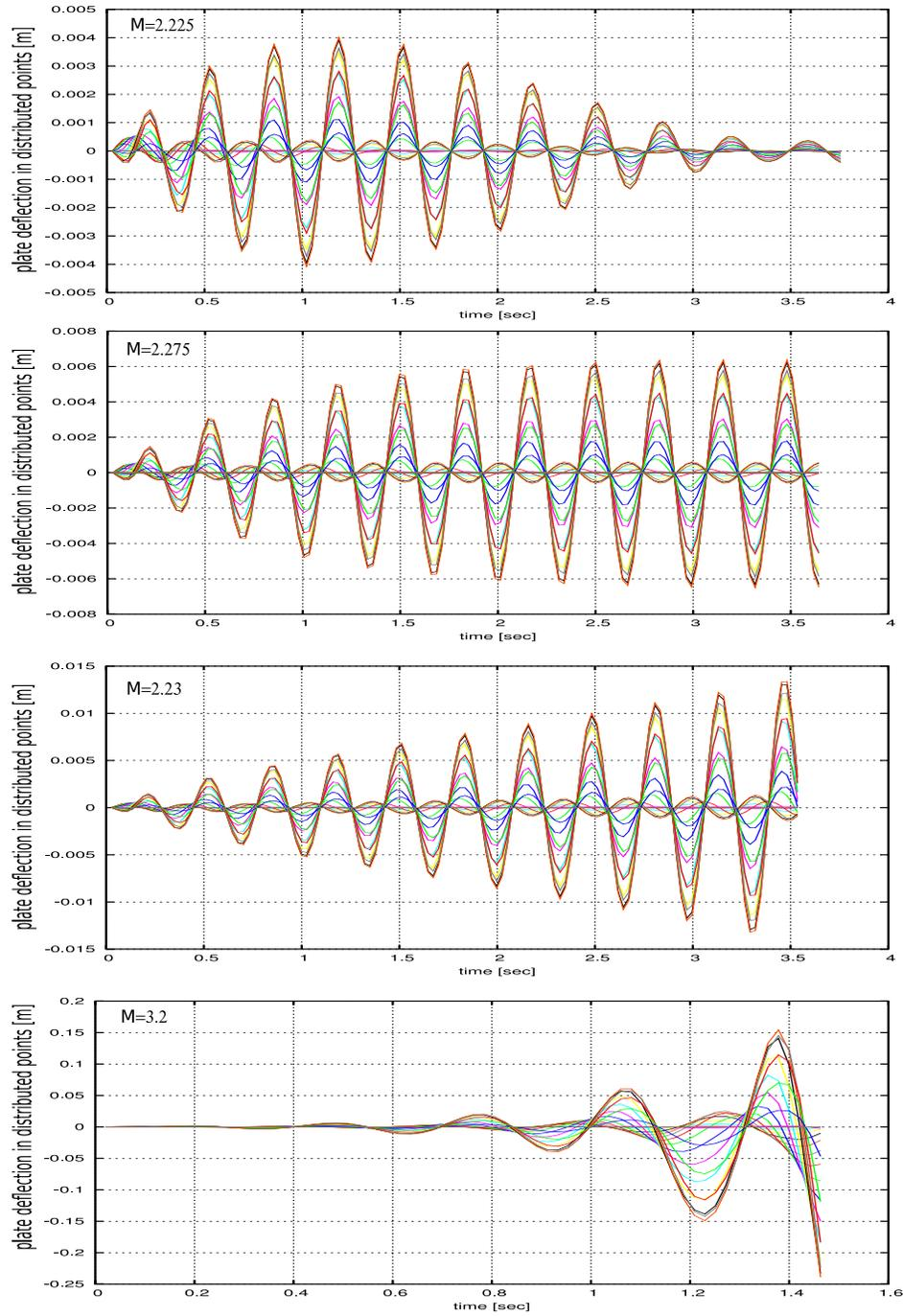
Figure 4: Plate deflection in distributed points along plate.
