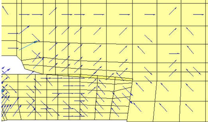
Figure 9: Directional refinement indicators for the coarse mesh.
