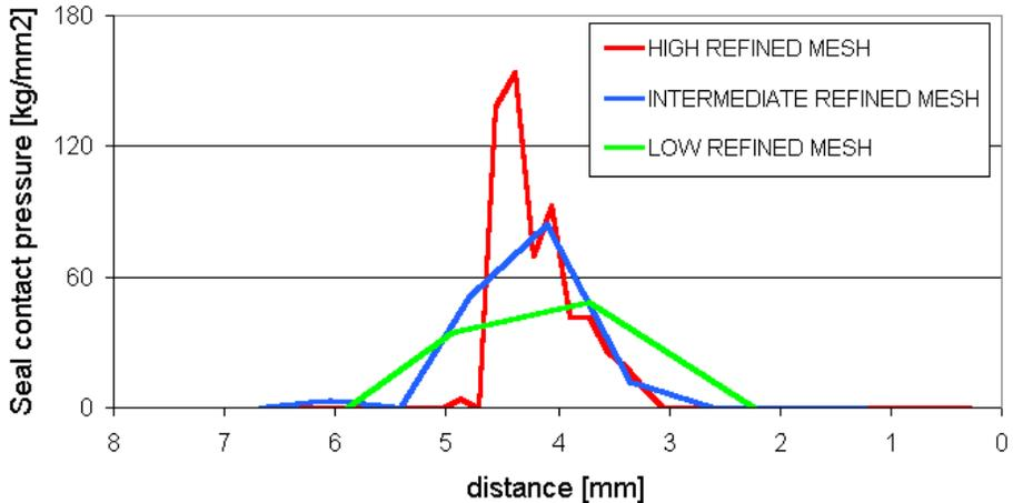
Figure 7: Variation of contact pressures with refinements.
