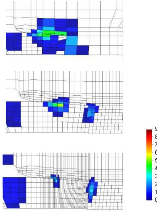
Figure 4: Refinement indicator for all the mesh. Detail in the region of the sealing.
