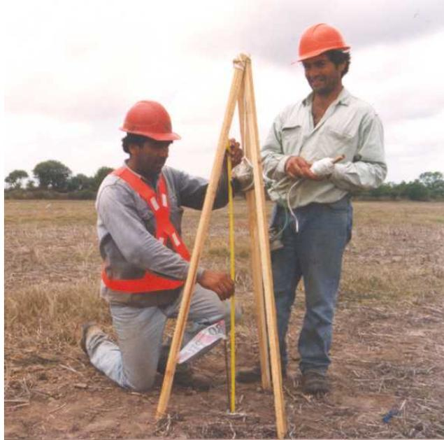
Figure 2: Elevated-charge support system
