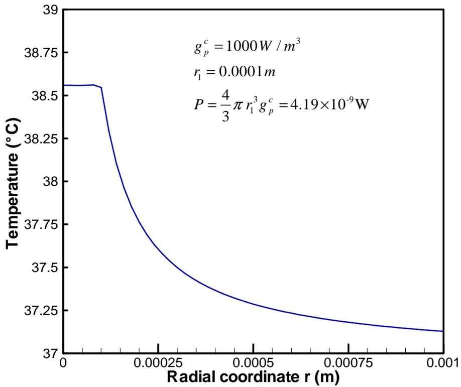
Figure 3 – Steady state temperature profile for  $r_1=0.0001 \text{ m}$
