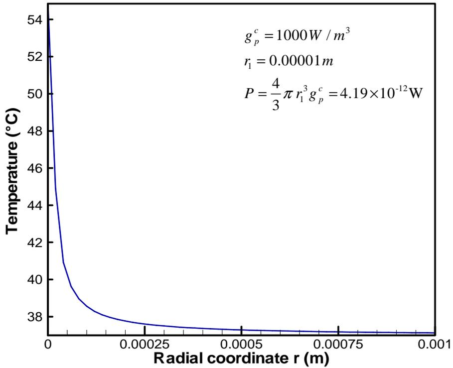
Figure 2 – Steady state temperature profile for  $r_1=0.00001 \text{ m}$
