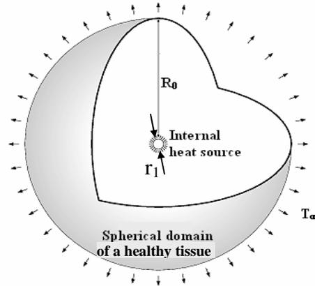
**Figure 1 – Schematic of the spherical domain with an internal heat source**
