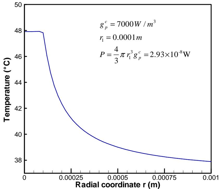
**Figure 4 – Steady state temperature profile for  $r_1=0.0001$  m and  $g_p^c=7000$  W/m<sup>3</sup>**
