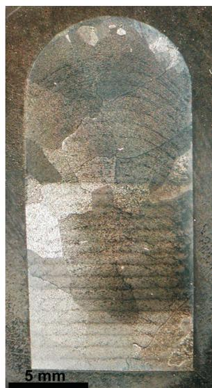
Figure 2: Etched cross section of specimen 05 obtained by SMD.
