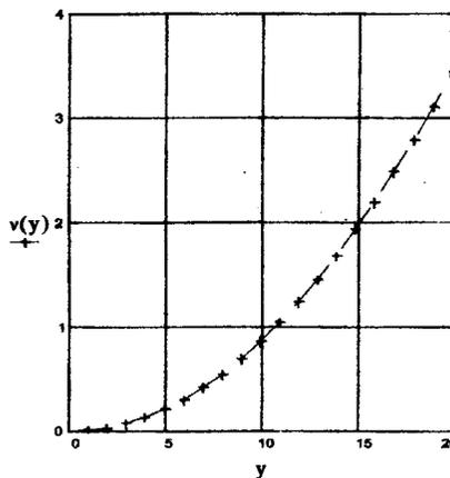
Figure 1. Non dimensional eddy viscosity in the near-wall region as a function of non dimensional wall distance
