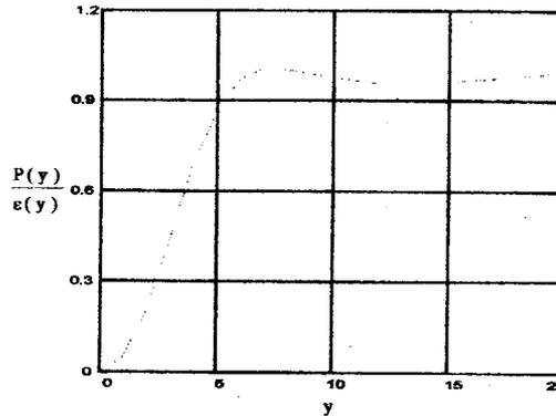
Figure 3. Relationship between dimensionless turbulent production and dissipation as a function of dimensionless wall distance
