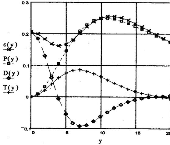
Figure 2. Near-wall behavior of turbulent dimensionless dissipation ( $\varepsilon^+$ ), viscous diffusion ( $D^+$ ), production ( $P^+$ ) and inertial transfer ( $T^+$ ), as a function of dimensionless wall distance ( $y^+$ ).
