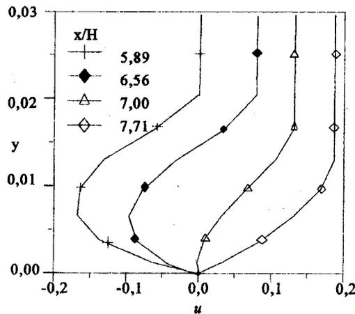
Figure 5. Mean velocity profile next to the reattachment point for the backward facing step problem
