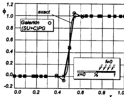
13: Example with internal source and null advection. Comparison between the different methods.
