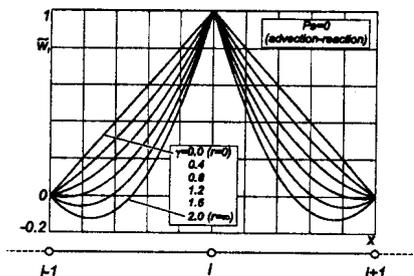
Figure 1: Weight functions for the null advection case.
