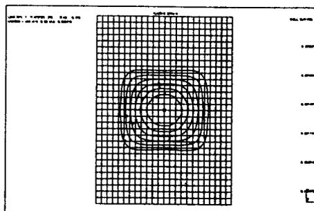
Fig. 4: Effective plastic strain at  $t = 0.375$  s in plasticity with hardening
