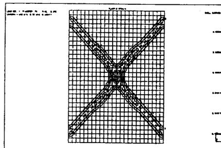
Fig. 2: Effective plastic strain field at  $t = 0.375$  s
