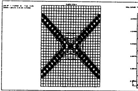
Fig. 9: Effective plastic strains at  $t = 0.375$  s with a relative permeability of  $K_w = 0.25E-03$  m/s
