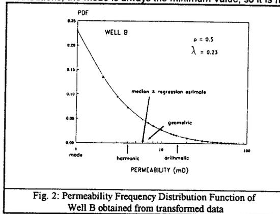
Fig. 2: Permeability Frequency Distribution Function of Well B obtained from transformed data
