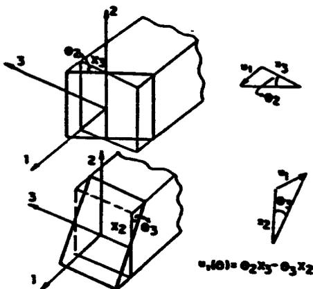
Figure 2. Displacements of a point in a cross section
