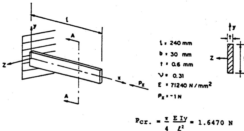
Figure 3. Axially Loaded Cantilever Beam.
