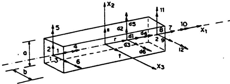
Figure 1. Linear Lagrangian Element
