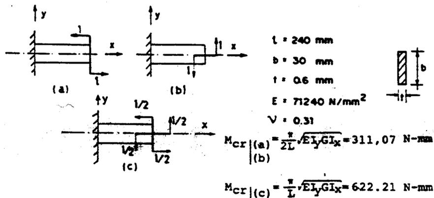
Figure 4. Cantilever with different load cases
