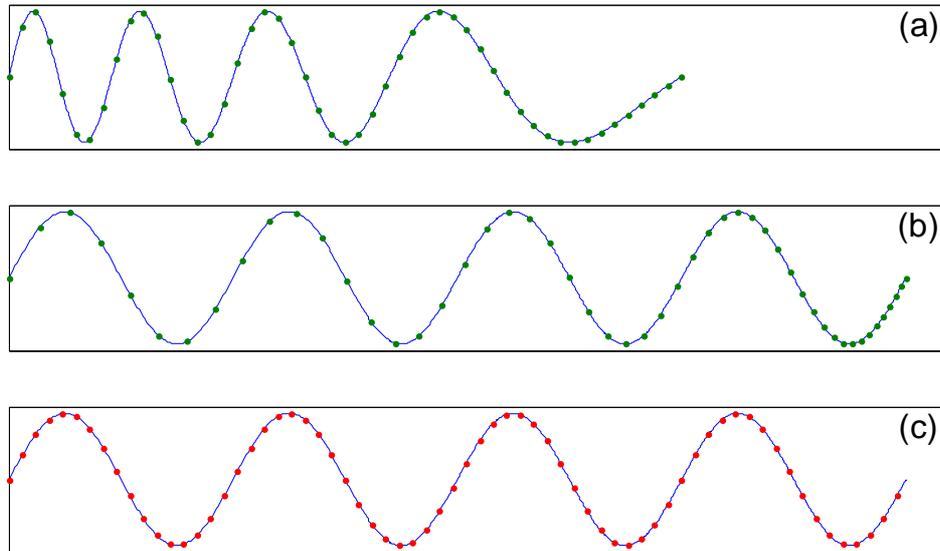
Figure 2: Pilot tone for illustrating Doppler compensation: (a) input signal and its equally spaced samples; (b) output signal and its non-uniformly spaced samples; (c) output signal uniformly sampled.
