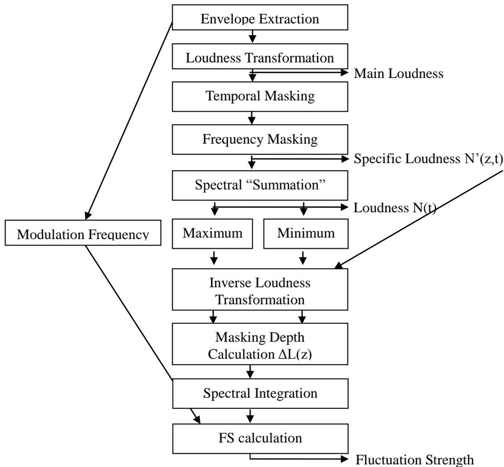
Figure 1: Fluctuation Strength calculation blocks diagram
