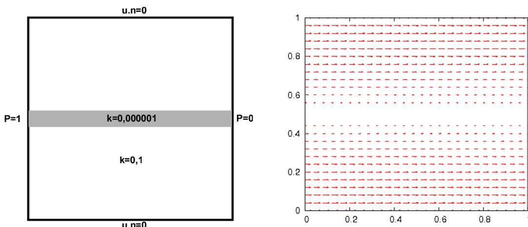
Figure 1: Heterogeneous Permeability — Domain and Results
