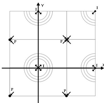
Figure 2: Configuration of a quarter of the five-spot pattern (Castro, 1999)
