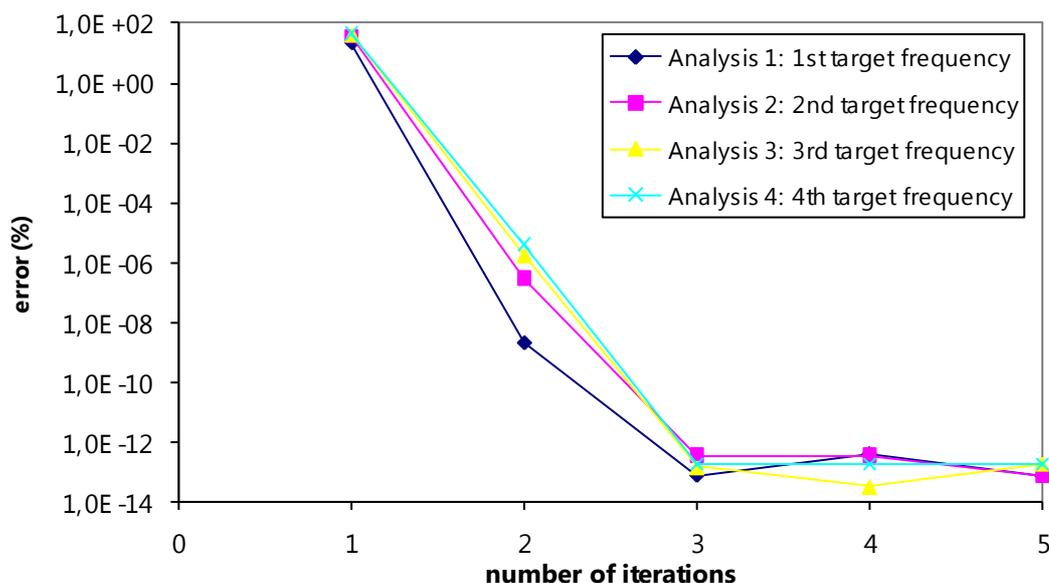
Figure 4: Relative error for the target eigenvalues – Uniform fixed-fixed bar
