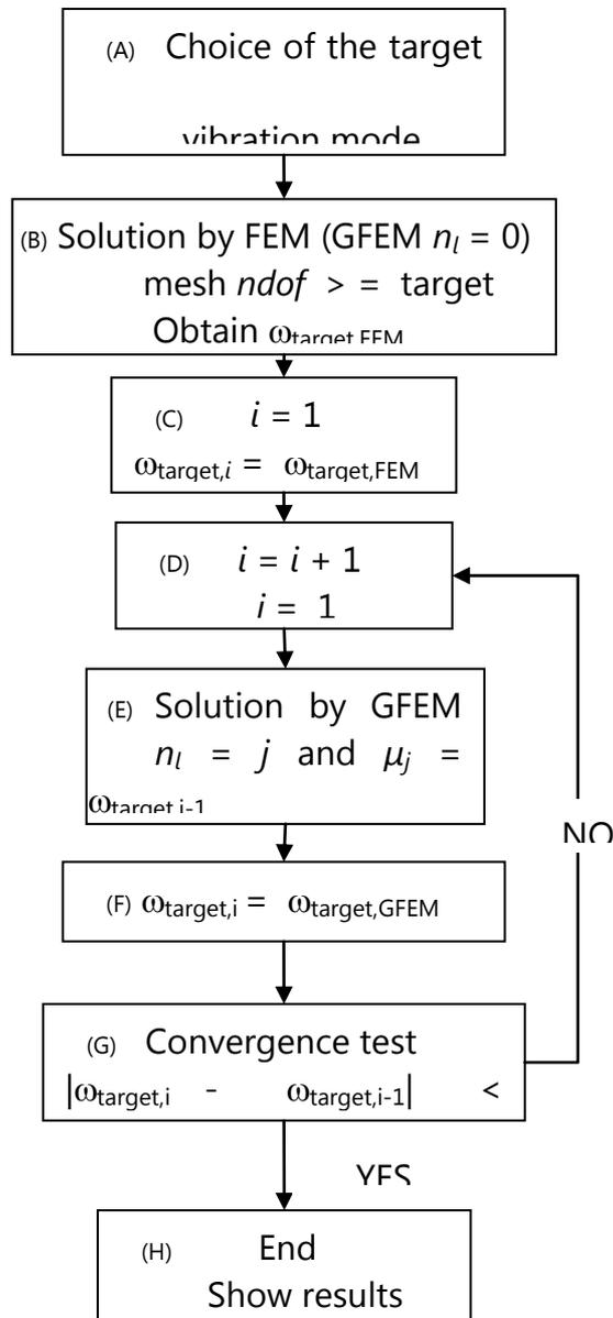
Figure 2: Flowchart of the adaptive Generalized Finite Element Method
