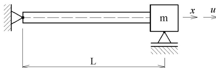
Figure 5: Uniform fixed-free bar carrying a concentrated mass
