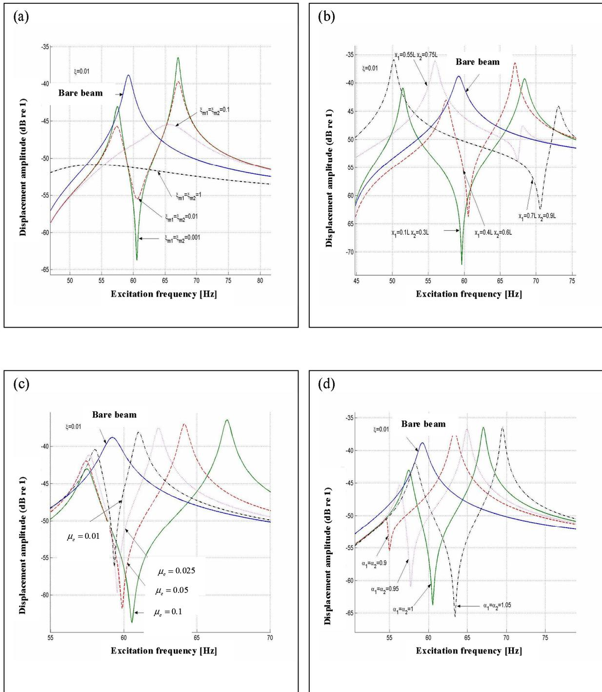
Figure 9: Frequency response curves of a beam with a 2-DOF system attached to it; frequencies near the second resonance of the beam.(a) Absorber with different damping coefficient; (b) at different locations; (c) with different mass ratios; (d) with different tuning ratios.
