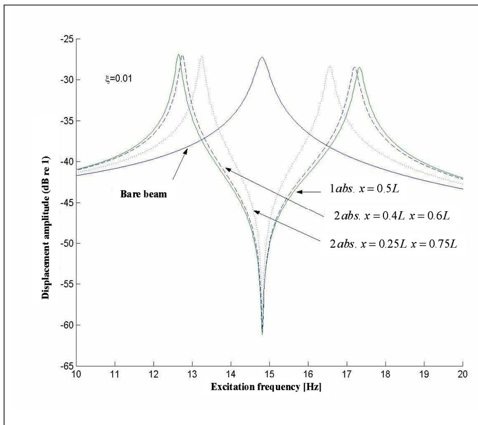
Figure 8: Frequency response of a beam with one 1-DOF system or two 1-DOF systems attached to it. The total mass of the two 1-DOF systems is equal to the mass of the 1-DOF system for a meaningful comparison.
