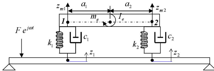
Figure 1: Schematic representation of the 2-DOF system attached to a beam.
