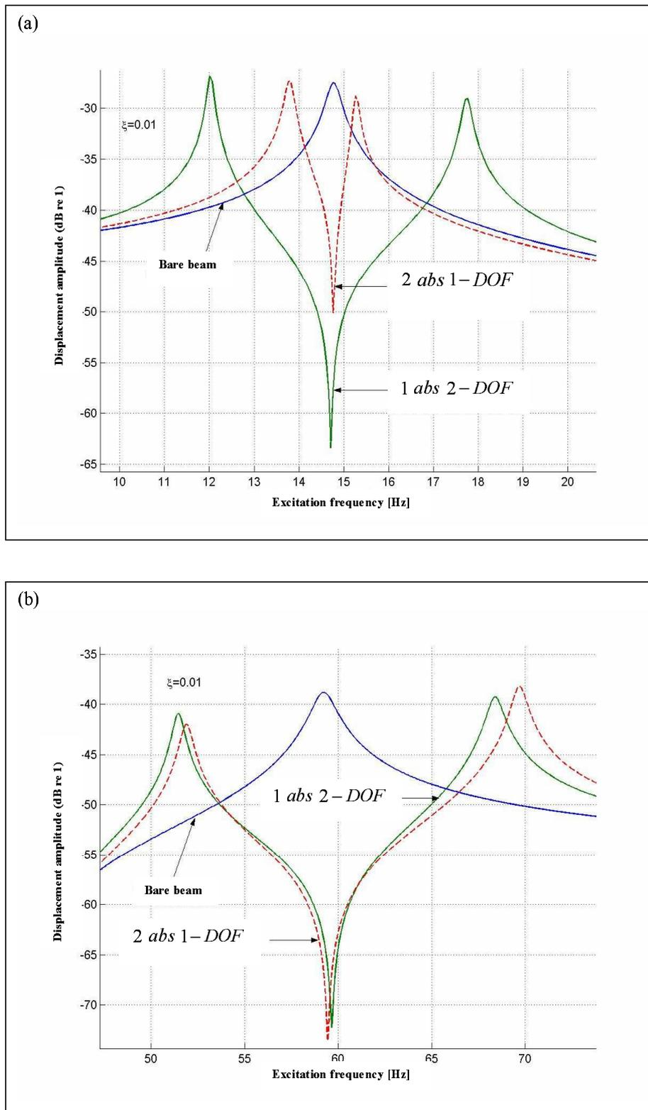
Figure 11: Frequency response of a beam with one 2-DOF system and two 1-DOF systems. Location of the absorbers:  $x_1 = 0.1L$  y  $x_2 = 0.3L$ . (a) Frequencies near the first resonance of the beam; (b) frequencies near the second resonance of the beam.
