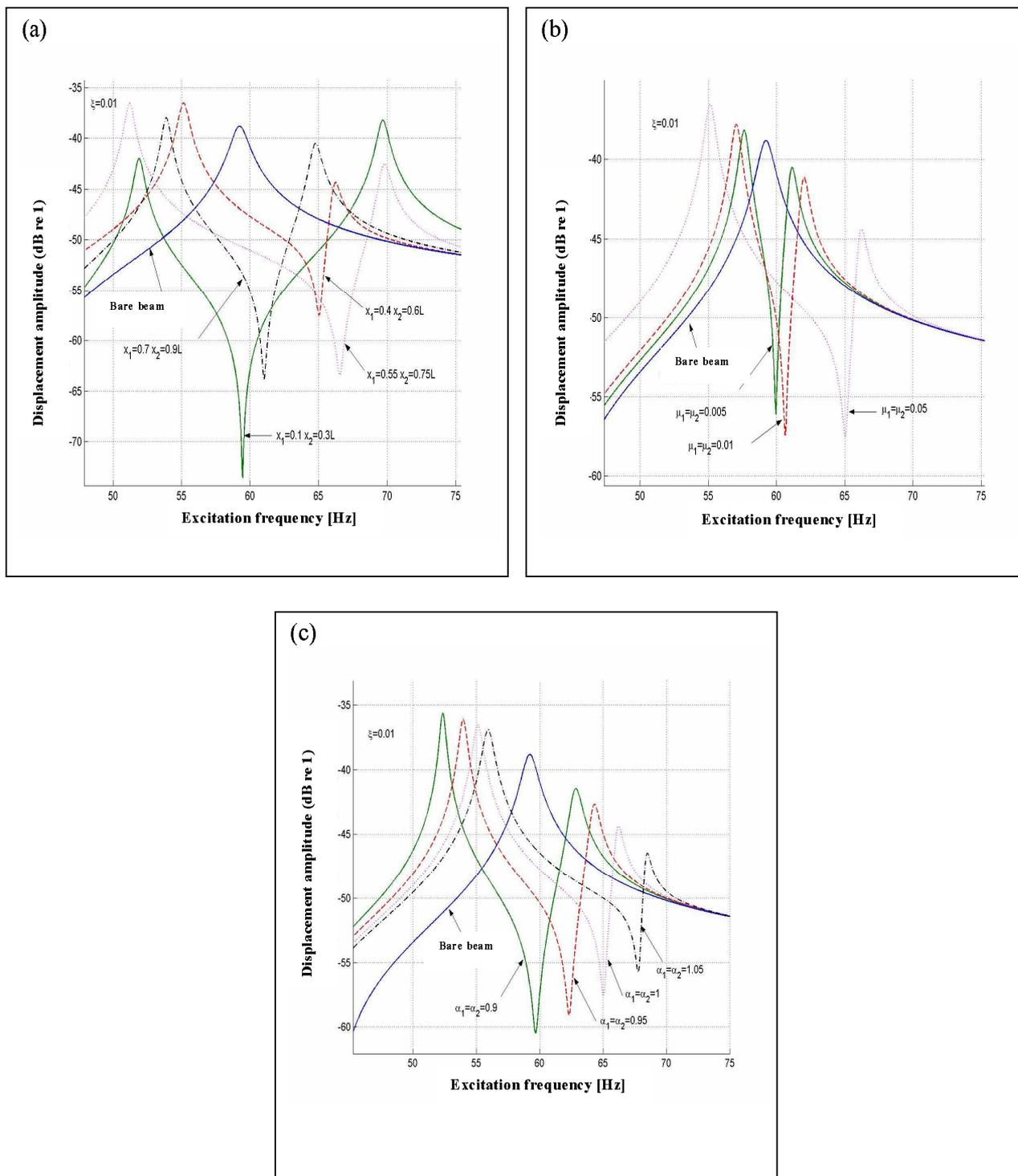
Figure 7: Frequency response of 2 1-DOF system attached to a beam. (a) Amplitudes for different locations of the absorbers, (b) for different mass ratios, (c) for different tuning ratios.
