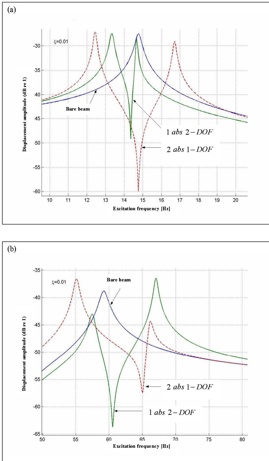
Figure 10: Frequency response of a beam with one 2-DOF system and two 1-DOF systems. Location of the absorbers  $x_1 = 0.4L$  y  $x_2 = 0.6L$ , (a) frequencies near the first resonance of the beam; (b) frequencies near the second resonance of the beam.
