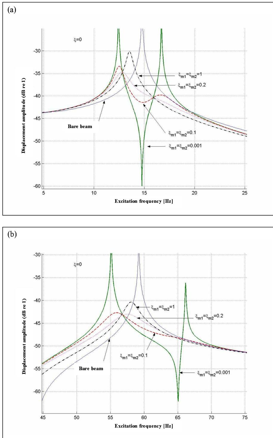
Figure 5: Frequency response of 2 1-DOF systems attached to an undamped beam ( $\xi = 0$ ). (a) Amplitudes near the first resonance of the beam;  $\mu_1 = \mu_2 = 0.05$ ,  $x_1 = 0.4L$ ,  $x_2 = 0.6L$ . (b) Idem (a) for amplitudes near the second resonance of the beam.
