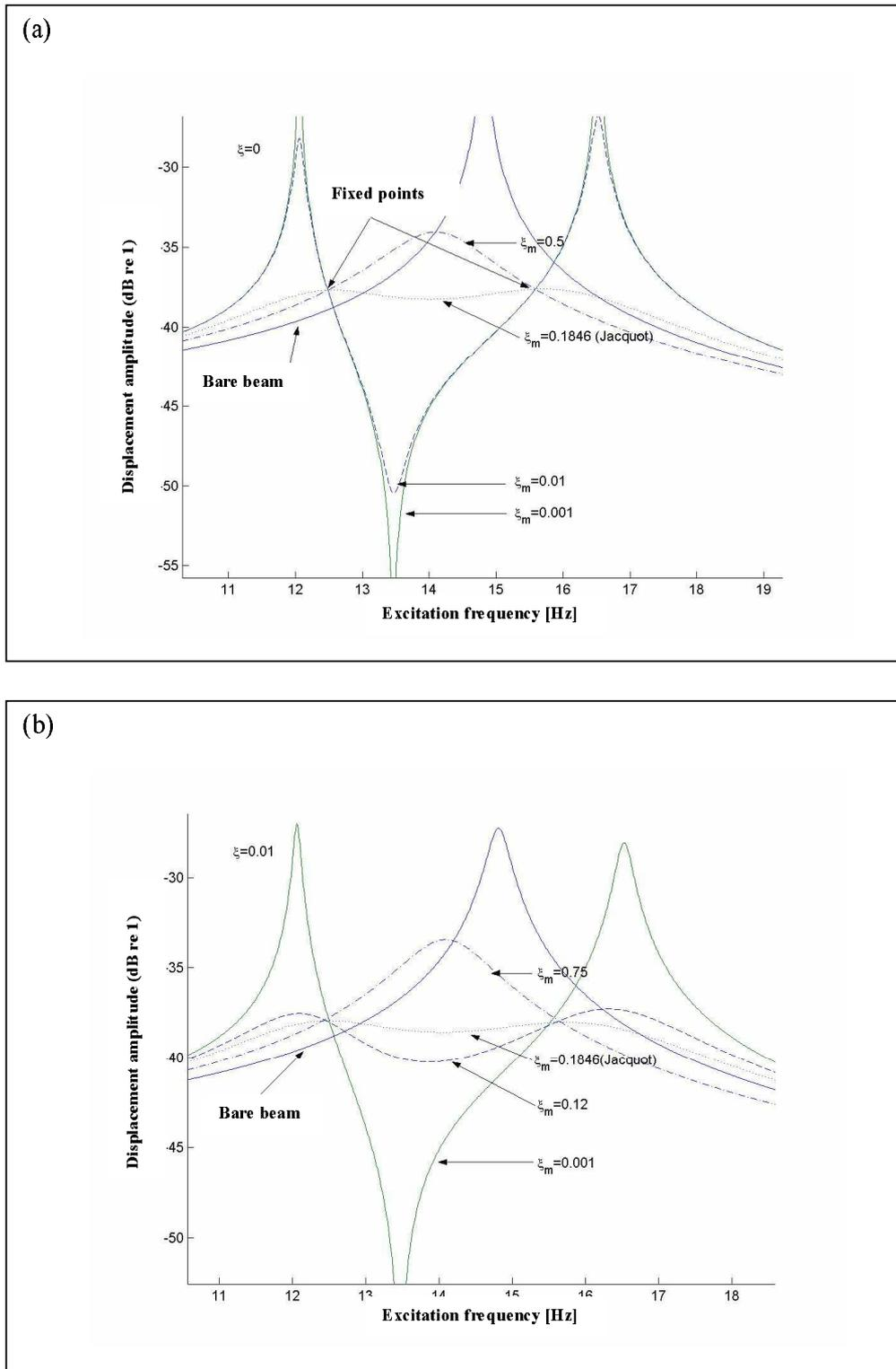
Figure 4: Frequency response of a 1-DOF system mounted to a beam. (a) Beam without damping ( $\xi = 0$ ),  $\mu = 0.05$ ,  $x_1 = 0.5L$  (b) idem (a) Beam with damping  $\xi = 0.01$ .
