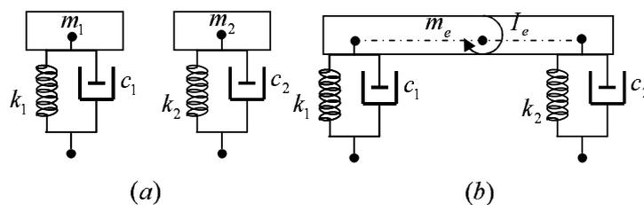
Figure 2: (a) Uncoupled 2-DOF system (2 1-DOF systems) and (b) coupled 2-DOF system.
