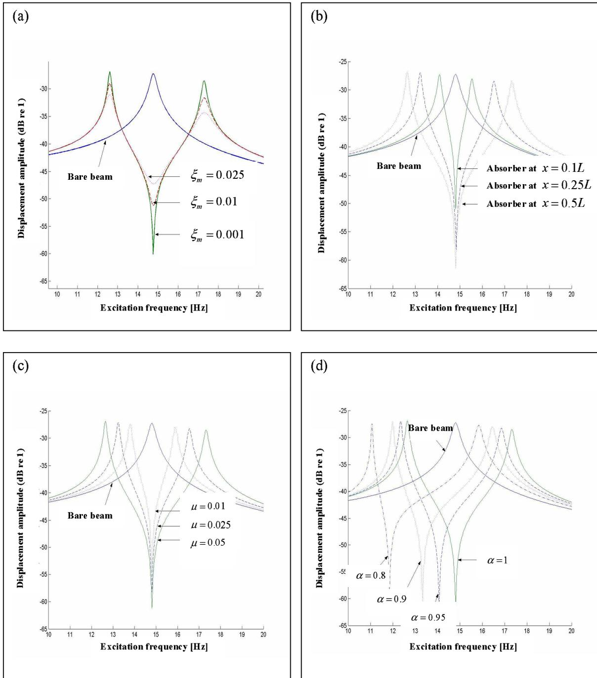
Figure 3: Frequency response of a 1-DOF system (absorber) attached to a beam. (a) absorber with different damping coefficients ( $\mu = 0.05$ ,  $x_1 = 0.5L$ ), (b) absorber at different locations ( $\mu = 0.05$ ,  $\xi_m = 0.001$ ), (c) absorber with different mass ratios ( $x_1 = 0.5L$ ,  $\xi_m = 0.001$ ), (d) absorber with different tuning ratios ( $\mu = 0.05$ ,  $x_1 = 0.5L$ ,  $\xi_m = 0.001$ ).
