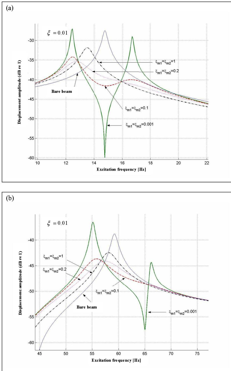
Figure 6: Frequency response of 2 1-DOF systems attached to a damped beam ( $\xi = 0.01$ ). (a) Amplitudes near the first resonance of the beam,  $\mu_1 = \mu_2 = 0.05$ ,  $x_1 = 0.4L$ ,  $x_2 = 0.6L$ . (b) Idem (a) amplitudes near the second resonance of the beam.
