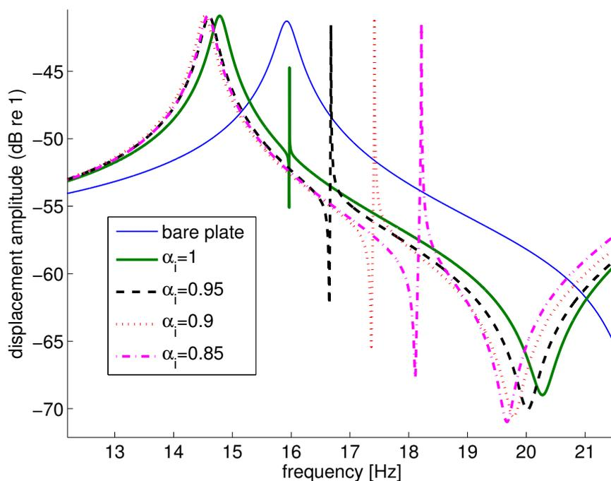
Figure 10: Displacement amplitude of a plate with a 3 DOF system for varying tuning ratio. Frequencies near the first resonance of the plate.
