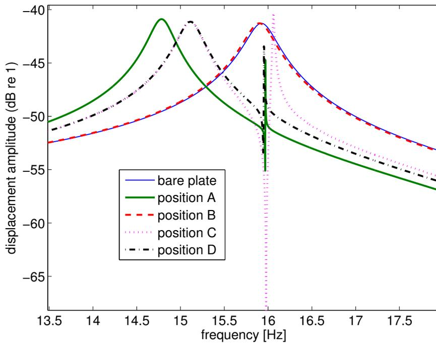
Figure 4: Displacement amplitude of a plate with a 3-DOF system for different locations of it. Frequencies near the first resonance of the plate.
