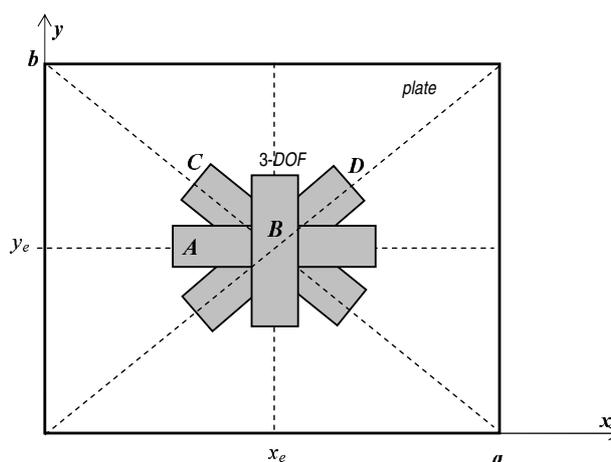
Figure 3: Different locations of the 3 DOF system on the plate to study the effect of its location on the dynamic behavior of the plate to which it is mounted.
