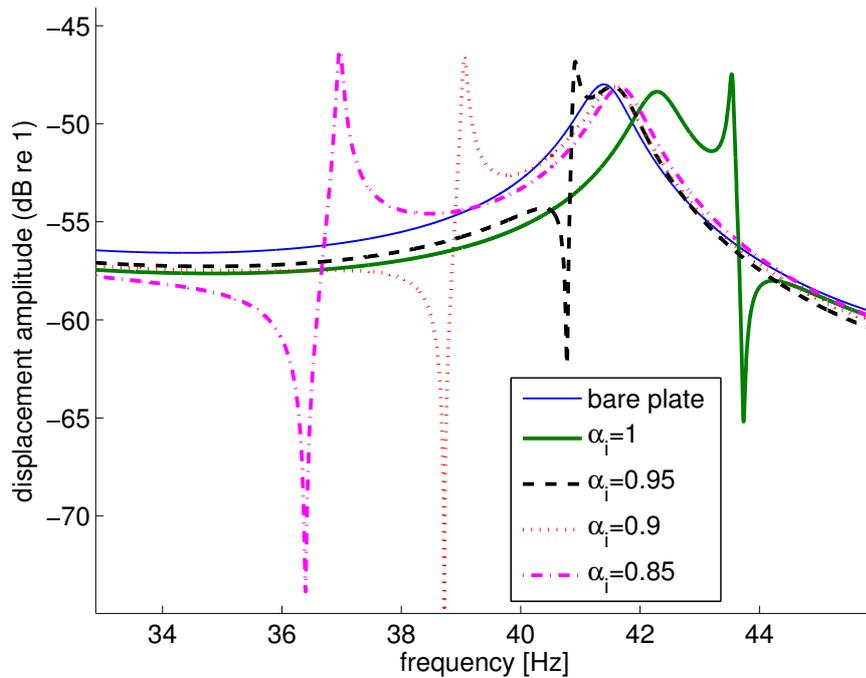
Figure 12: Idem Fig. 10. Frequencies near the third resonance of the plate
