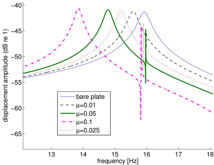
Figure 7: Displacement amplitude of a plate with a 3 DOF system for varying mass ratio. Frequencies near the first resonance of the plate.
