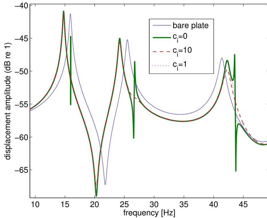
Figure 2: Displacement amplitude of a plate with a 3-DOF system for varying damping constant of the 3-DOF.
