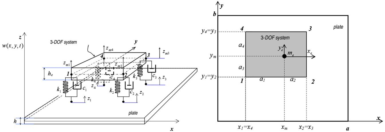
Figure 1: (a) Plate with a three degree-of-freedom DVA attached to it. (b) Nomenclature for the coordinates selected to describe the motion of the 3 DOF DVA.
