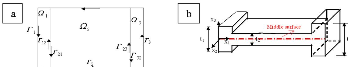
Figure 1: a) General zoned plate domain; b) Reference surface view.
