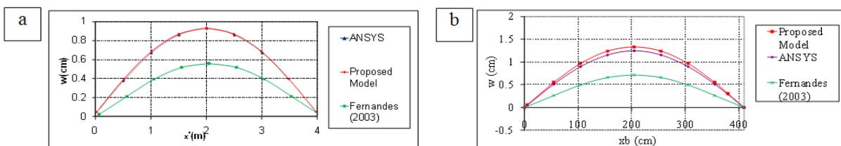
Figure 4 – a) Deflections along the plate axis  $X'$ b) Deflections along the beam axis  $X_b$
