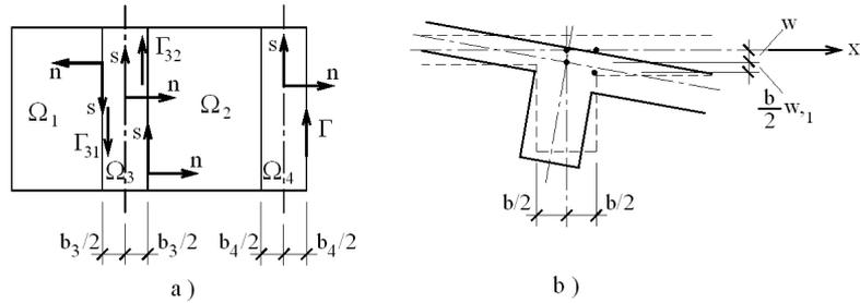
Figure 2: (a) Reinforced plate view; (b) Deflections approximations along interfaces
