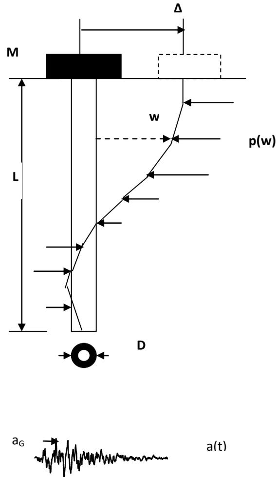
Figure 6. Pile steel tube under earthquake excitation
