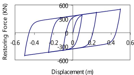
Figure 9. BWBN-developed loop for cyclic displacement history
