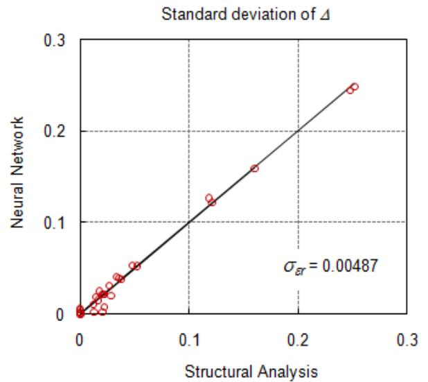
Figure 11. Neural network representation, standard deviation of the response
