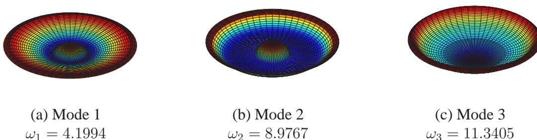
Figure 5: Axisymmetric structural modes of the conical shell configuration.
