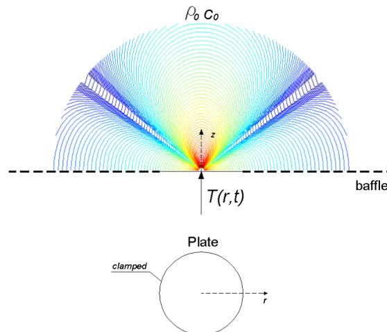
Figure 1: Model for the Acoustic-Plate Coupling.
