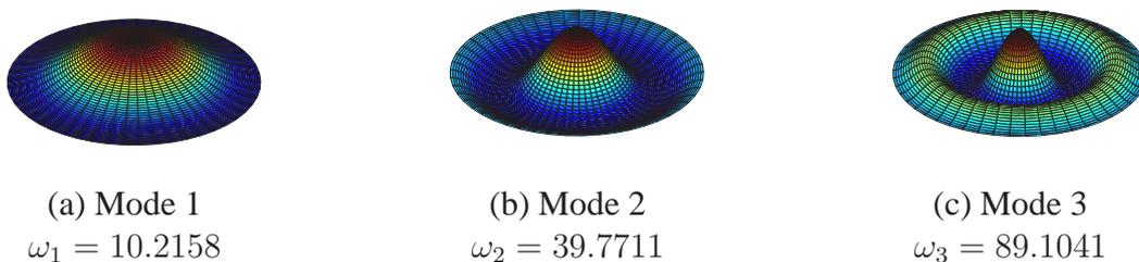
Figure 4: Axisymmetric structural modes of the flat plate configuration.
