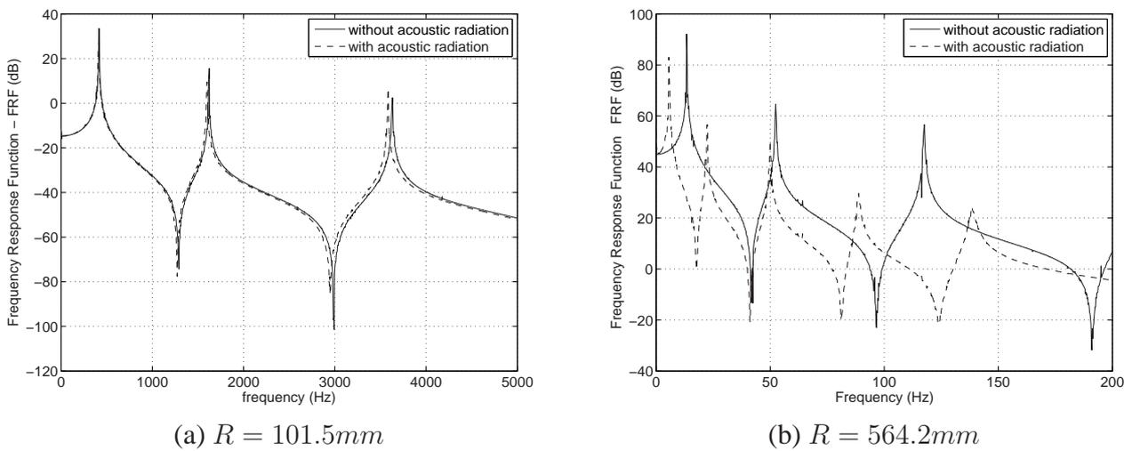
Figure 7: Frequency Response Functions of the flat plate.
