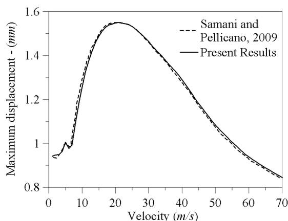
Figure 2 - Beam subjected to moving load and connected to linear fixed damper. Maximum displacement at mid-span of the L4 beam as a function of the load velocity.
