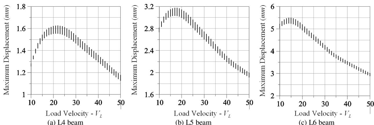
Figure 6 - Maximum displacement at mid-span of the beam ( $x = 0.5L$ ) versus load velocity ( $V_L$ ). (a) L4 beam, (b) L5 beam and (c) L6 beam.
