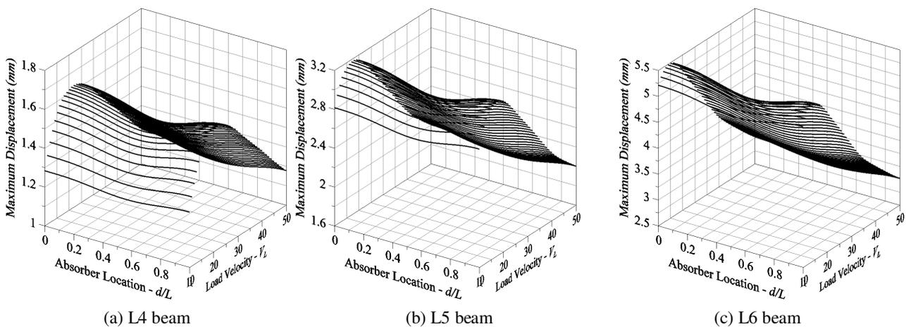
Figure 5 - Maximum displacement at mid-span of the beam ( $x = 0.5L$ ) as a function of the absorber location ( $d/L$ ) and load velocity ( $10 \leq V_L \leq 50$ ). (a) L4 beam, (b) L5 beam and (c) L6 beam.
