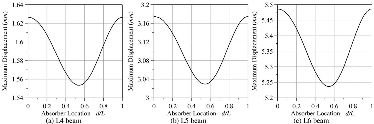
Figure 8 – Maximum beam displacement with varying absorber position. (a) L4 beam, (b) L5 beam and (c) L6 beam.
