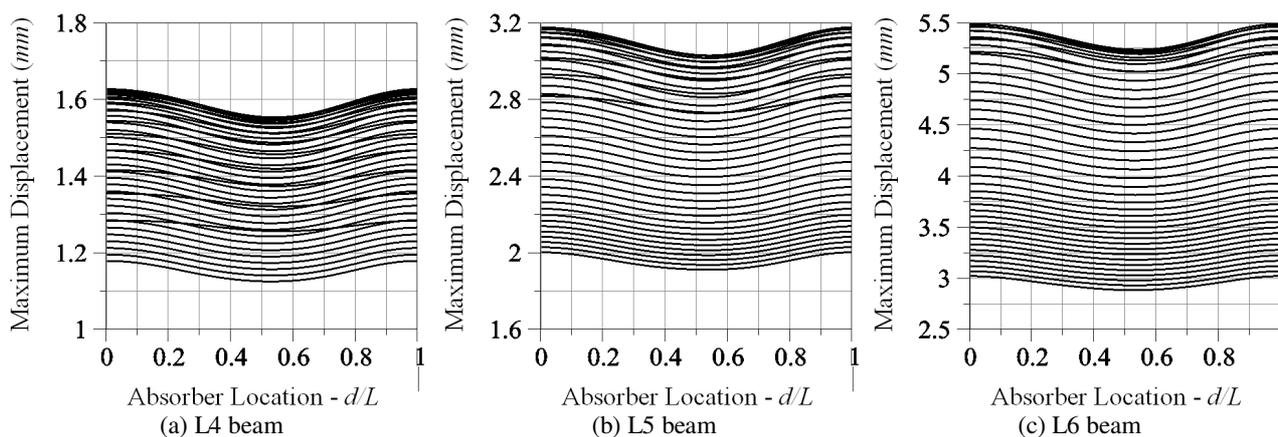
Figure 7 - Maximum displacement at mid-span of the beam ( $x = 0.5L$ ) as a function of the absorber location ( $d/L$ ). (a) L4 beam, (b) L5 beam and (c) L6 beam.
