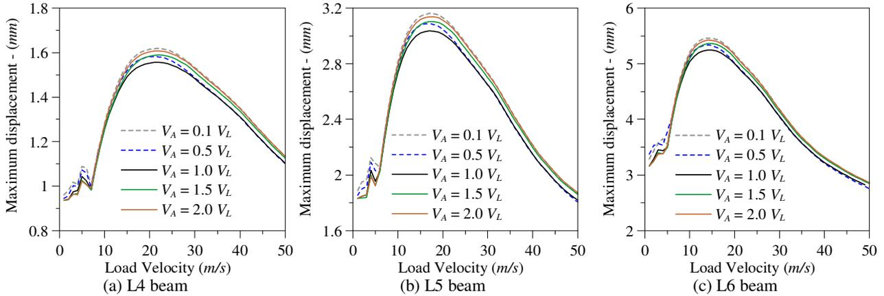
Figure 10 - Maximum displacement at mid-span of the beams ( $x = 0.5L$ ) versus Load velocity ( $V_L$ ). (a) L4 beam, (b) L5 beam and (c) L6 beam.
