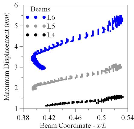
Figure 9 – Maximum beam displacement and coordinate at which it occurs for different absorber position ( $0 \leq d \leq L$ ) and load velocity varying in the interval  $10 \text{ m/s} \leq V_L \leq 50 \text{ m/s}$ .
