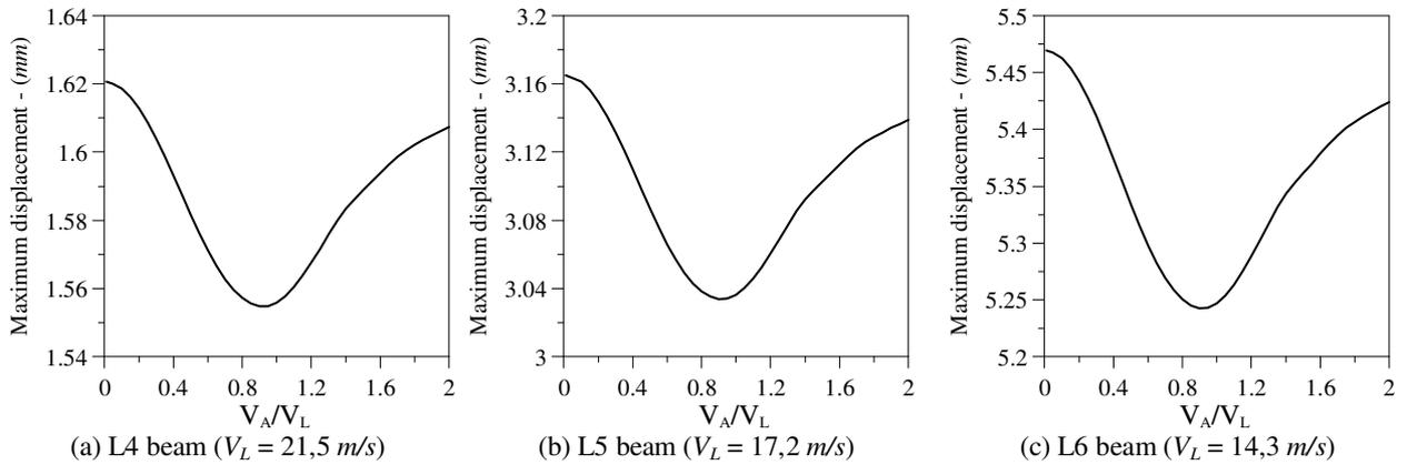
Figure 11 – Maximum displacement at mid-span as a function of  $V_A/V_L$ . (a) L4 beam, (b) L5 beam and (c) L6 beam.
