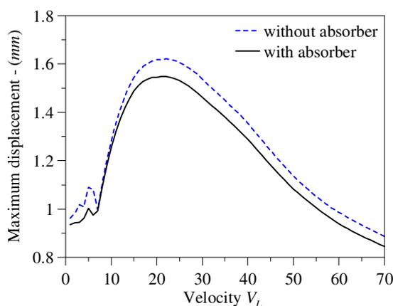
Figure 3 - Comparison maximum displacement at mid-span of the beam ( $x = 0.5L$ ). Beam L4 with and without absorbers.
