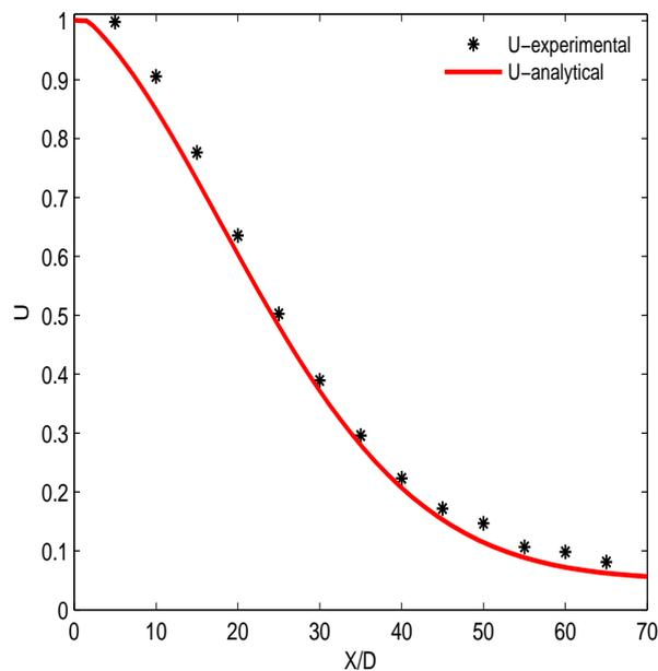
Figure 2: Comparison of the axial velocity for  $H_2/N_2$  jet with experiment ([Sandia National Laboratories, 2010](#)).
