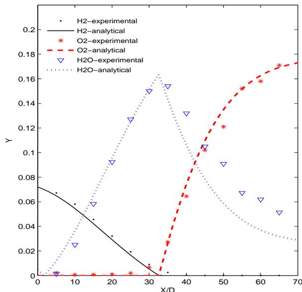
Figure 3: Mass fraction of fuel  $H_2$ , oxidizer  $O_2$ , and water vapor  $H_2O$  along the burner centerline.
