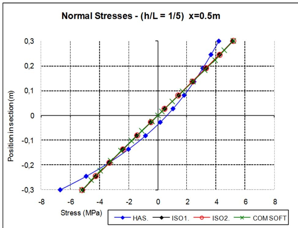
Figure 6: Normal Stresses –  $h/L=1/5$ ,  $x=0.5m$
