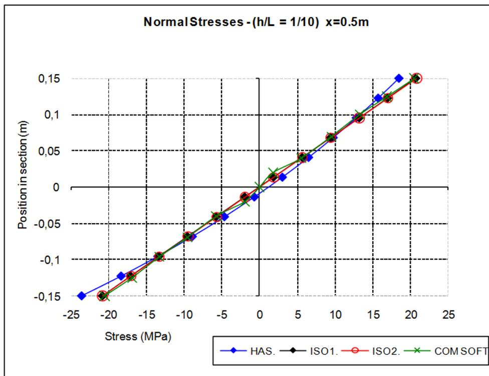
Figure 4: Normal Stresses –  $h/L=1/10$ ,  $x=0.5m$
