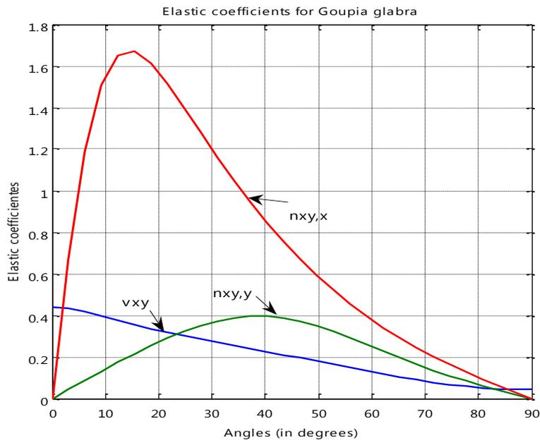
Figure 8: Elastic Coefficients for *Goupia glabra* –  $n_{xy,x}$ ,  $n_{xy,y}$ ,  $v_{xy}$ .
