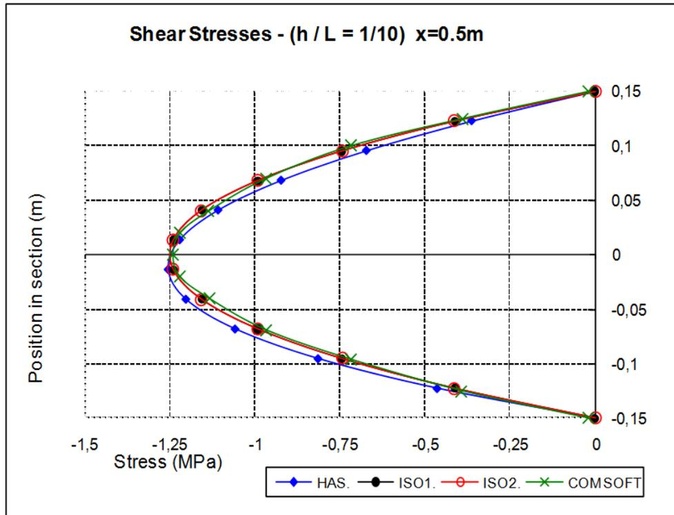
Figure 5: Shear Stresses –  $h/L=1/10$ ,  $x=0.5m$
