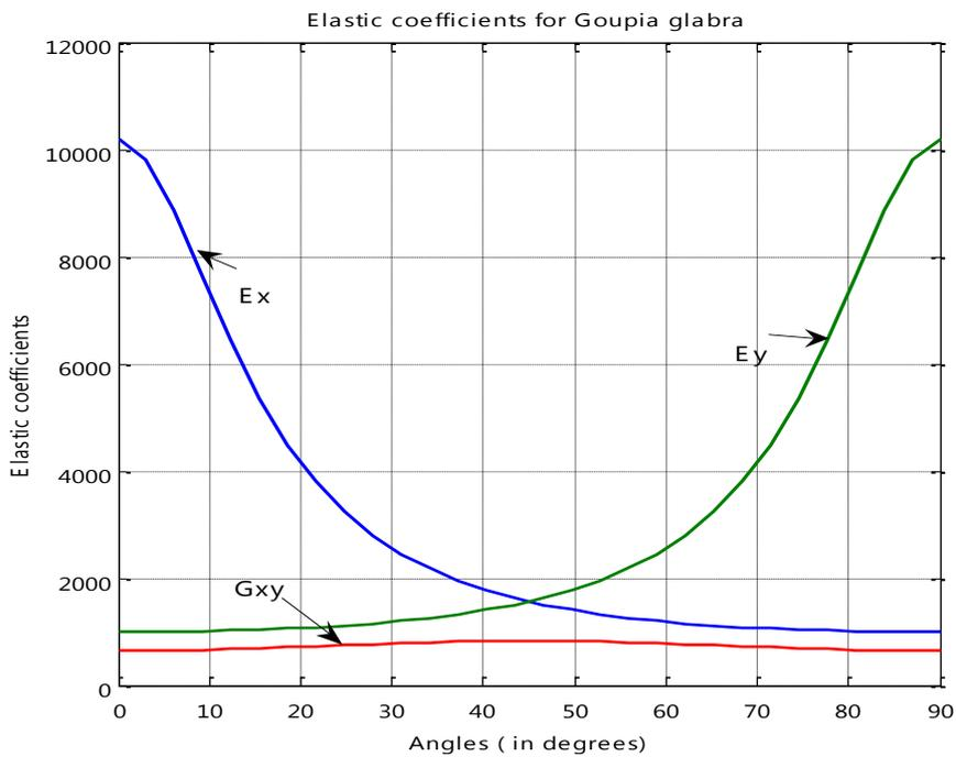
Figure 9: Elastic Coefficients for *Goupia glabra* –  $E_x$ ,  $E_y$ ,  $G_{xy}$ .
