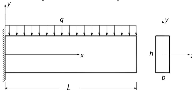
Figure 3: Wood Cantilever Beam
