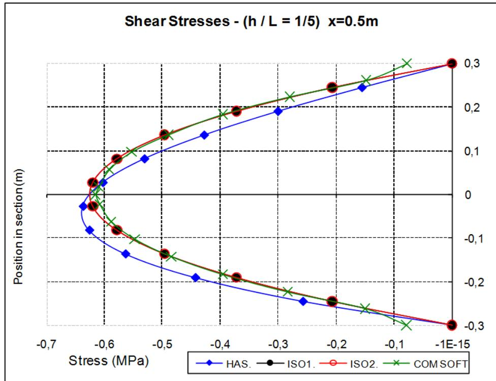
Figure 7: Shear Stresses –  $h/L=1/5$ ,  $x=0.5m$
