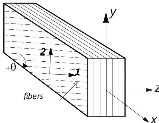
Figure 2: Wood Laminated Cantilever Beam
