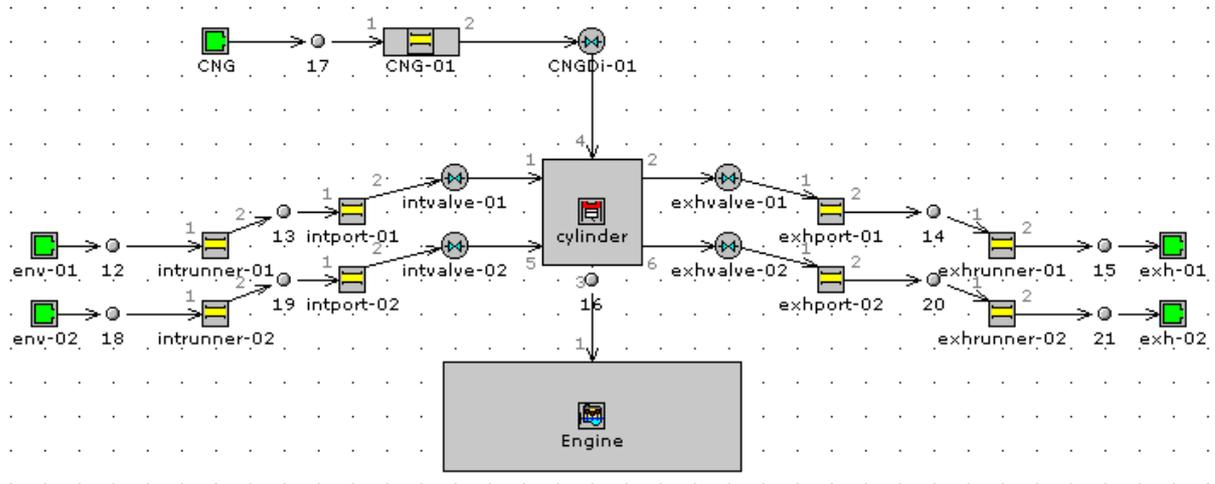
Figure 2 - Engine model using GT-POWER
