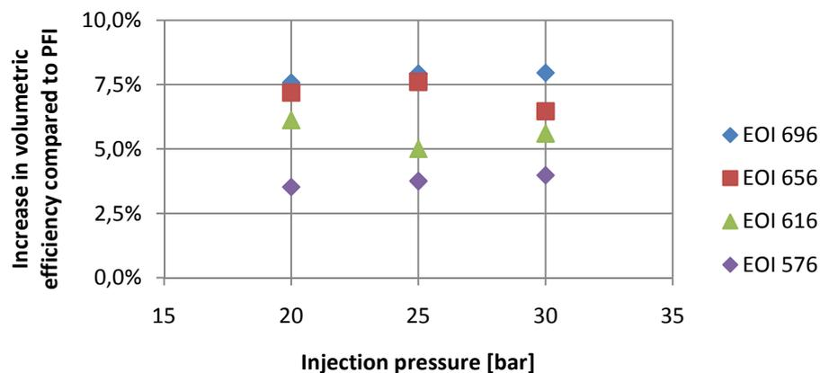
Figure 9 - Volumetric efficiency for different injection pressures keeping EOI constant
