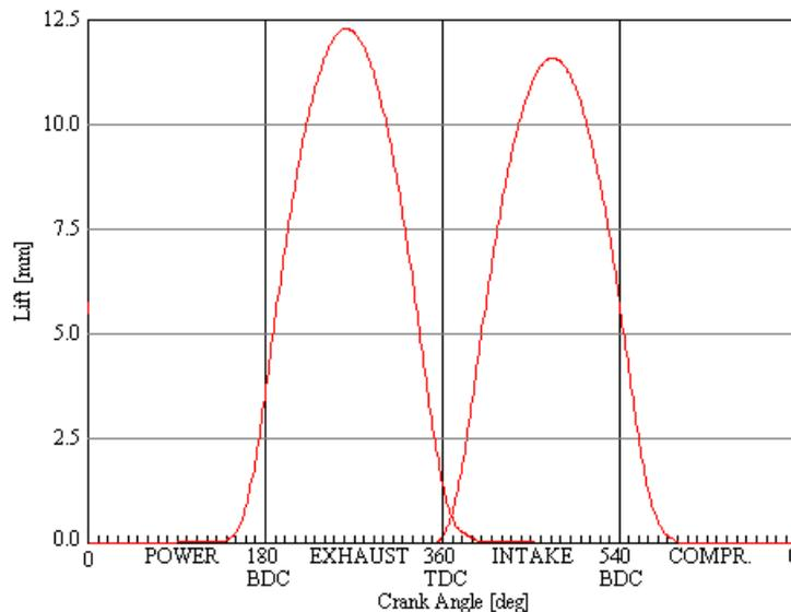
Figure 3 – Valve lift profiles
