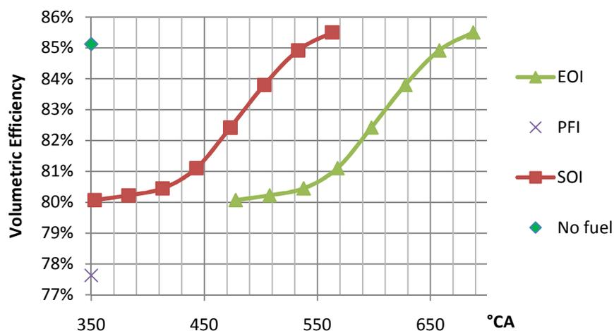
Figure 6 - Injection timing effect on volumetric efficiency
