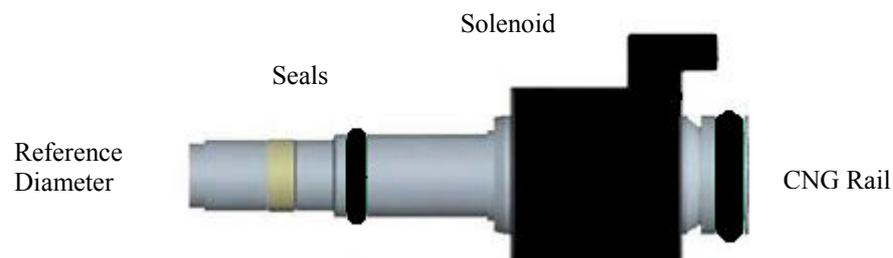
Figure 5 - CNG injector
