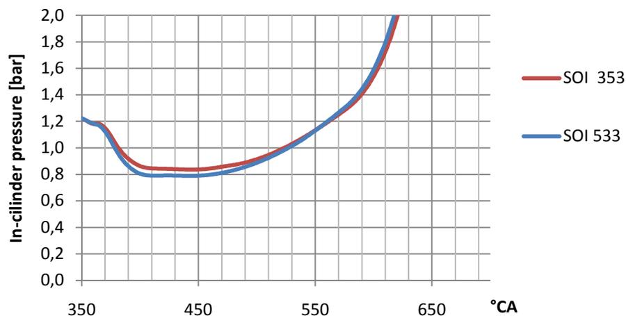
Figure 7 - In-cylinder pressure for different start of injection
