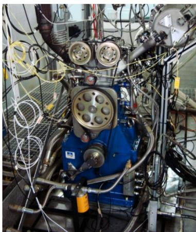
Figure 1 - Single cylinder research engine
