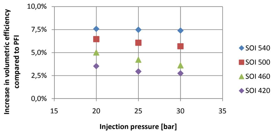
Figure 8 - Volumetric efficiency for different injection pressures and timings
