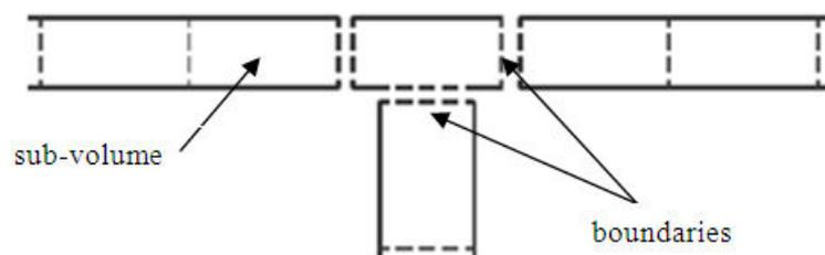
**Figure 4 – Component discretization**
