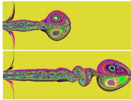
Figure 3: Starting and trailing vortex dipoles from two-dimensional direct numerical simulations at different stages of the flow through a single slit larynx-shaped channel.
