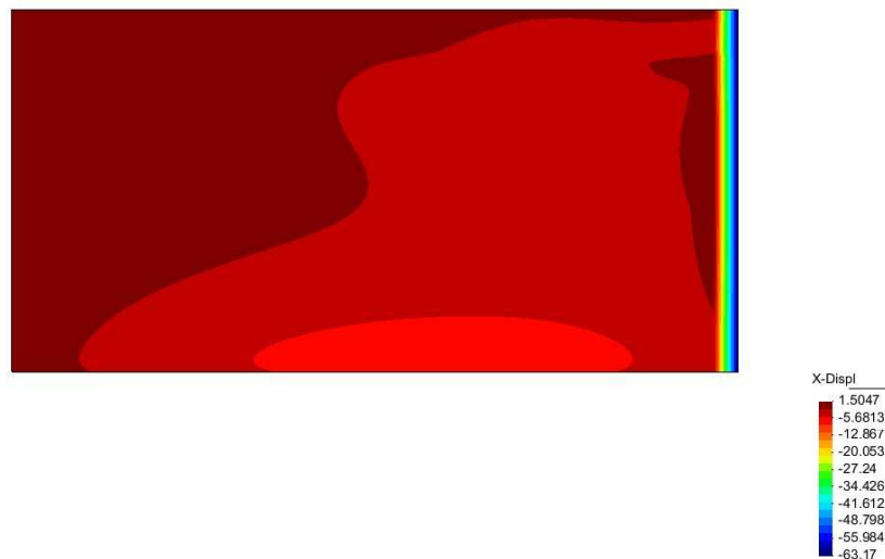
Figure 14: Contours fill of total horizontal displacement at failure \Delta t = 126000 years.
