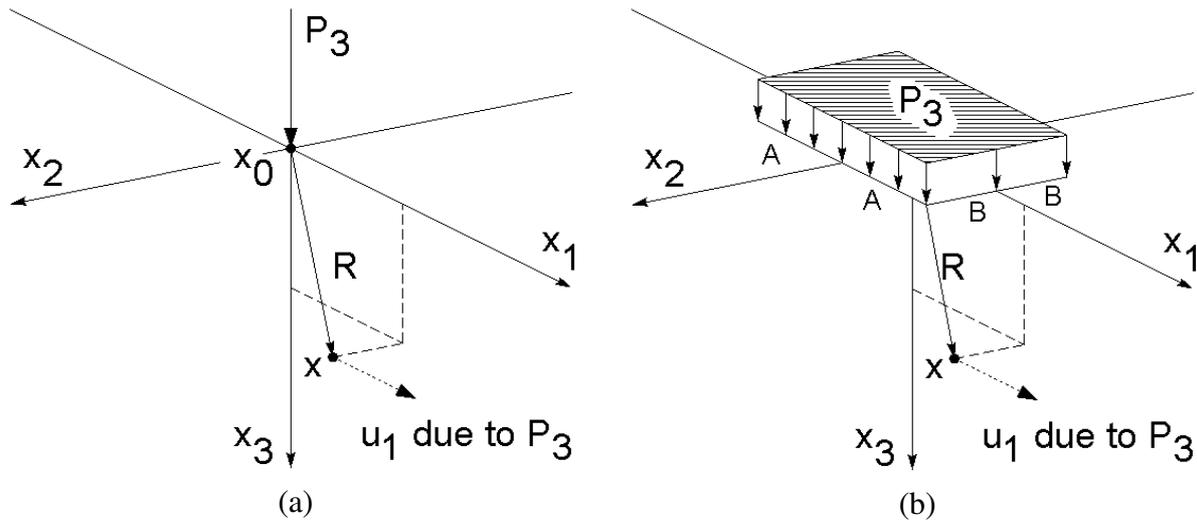
Figure 1: Examples of Green's functions of the displacement field of a 3D space, due to (a) concentrated and (b) distributed loads.
