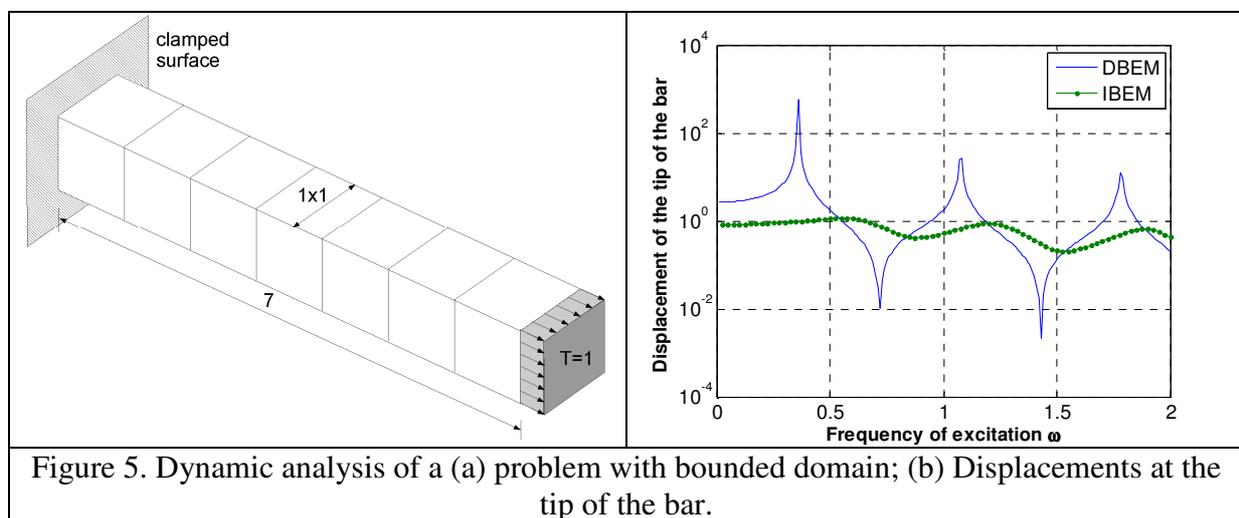
The problem consists of a long 3D bar, discretized by 30 square boundary elements. One of its ends is clamped, and the other end is subjected to a uniformly distributed harmonic load of unitary intensity. The material parameters are: Poisson's ratio  $\nu=0.25$ ; Lamé's constant  $\mu=1.0$ ; Young's modulus  $E=2.5$ .
