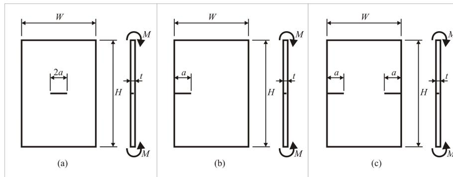
Figure 1: Geometry (a) Central cracked plate. (b) A single edge-cracked plate. (c) Double edge cracked plate.
