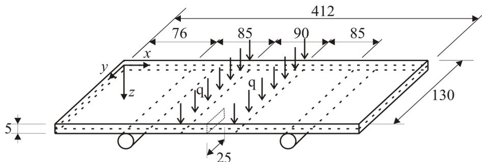
Figure 8: Detailed sketch of plate dimensions.
