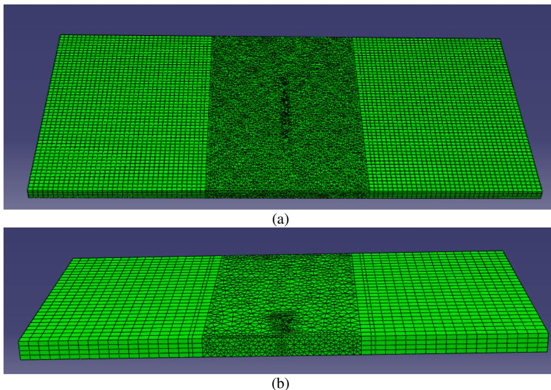
Figure 2: Mesh (a) Central cracked plate,  $t = 5$  mm. (b) A single edge-cracked plate,  $t = 10$  mm.
