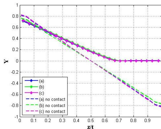
Figure 6: Normalized stress intensity factor along the crack front ( $t = 20$  mm): (a) Central cracked plate. (b) A single edge cracked plate. (c) Double edge cracked plate
