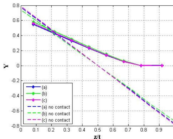
Figure 4: Normalized stress intensity factor along the crack front ( $t = 5$  mm): (a) Central cracked plate. (b) A single edge cracked plate. (c) Double edge cracked plate.
