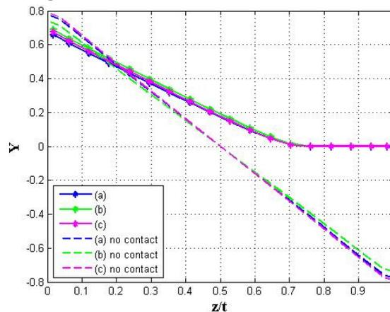
Figure 5: Normalized stress intensity factor along the crack front ( $t = 10$  mm): (a) Central cracked plate. (b) A single edge cracked plate. (c) Double edge cracked plate.
