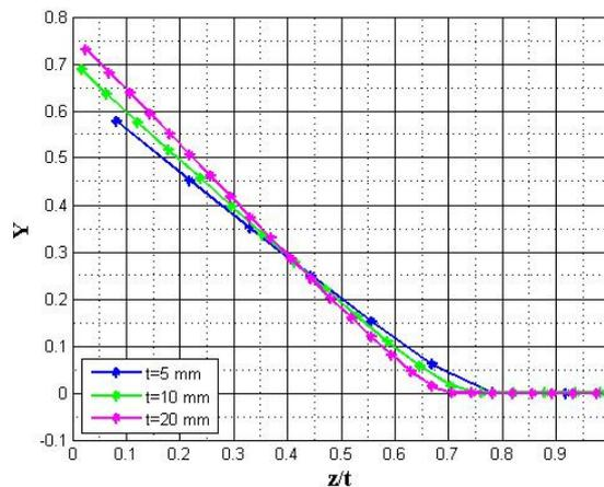
Figure 7: Normalized stress intensity factor for various thicknesses along the crack front of a single edge cracked plate.
