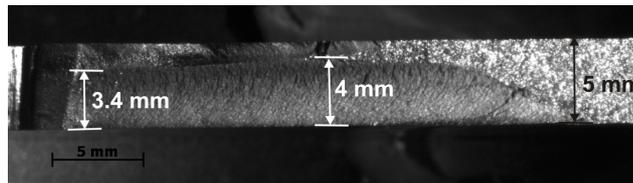
Figure 10: View of the growth crack.
