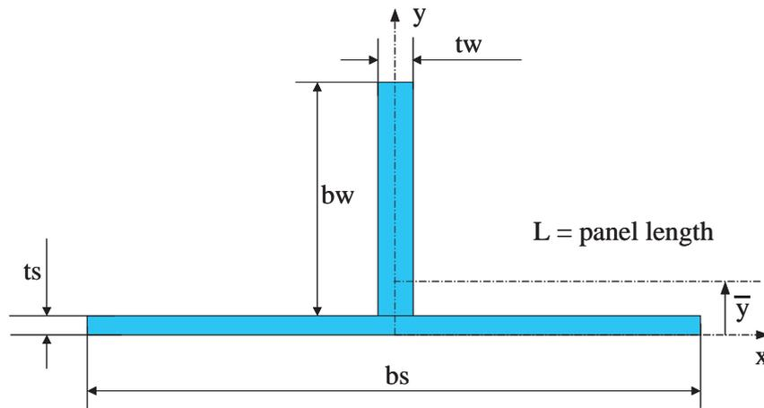
Figure 6: Panel geometry.
