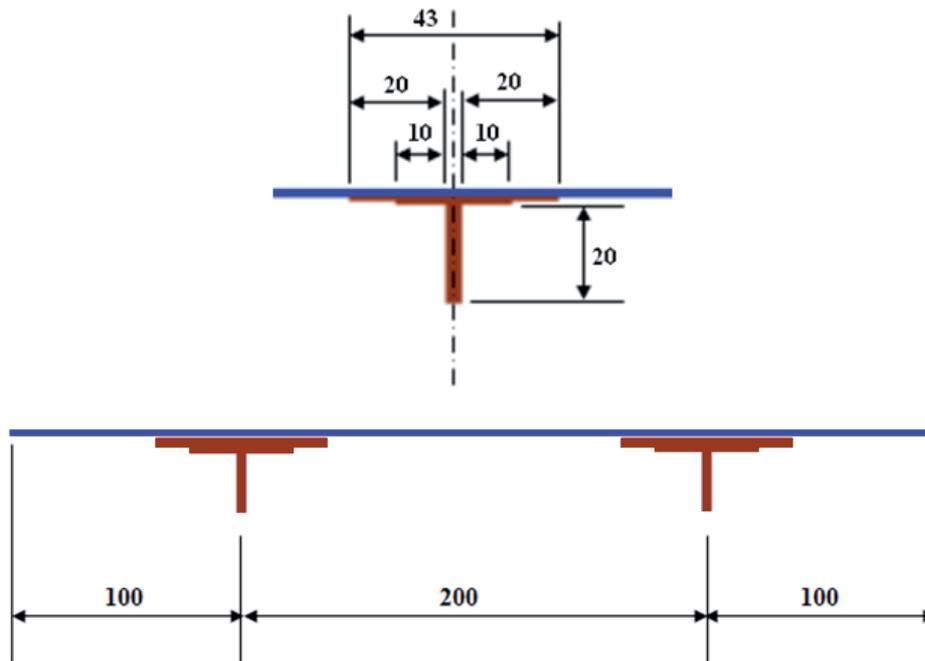
Figure 2: Stiffener section and panel dimensions (in mm).
