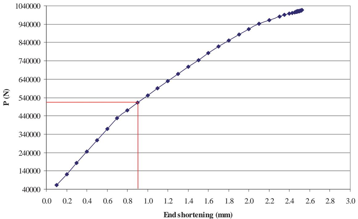
Figure 10: Non linear solution results for the composite panel with the optimal dimensions of Neto (2006).
