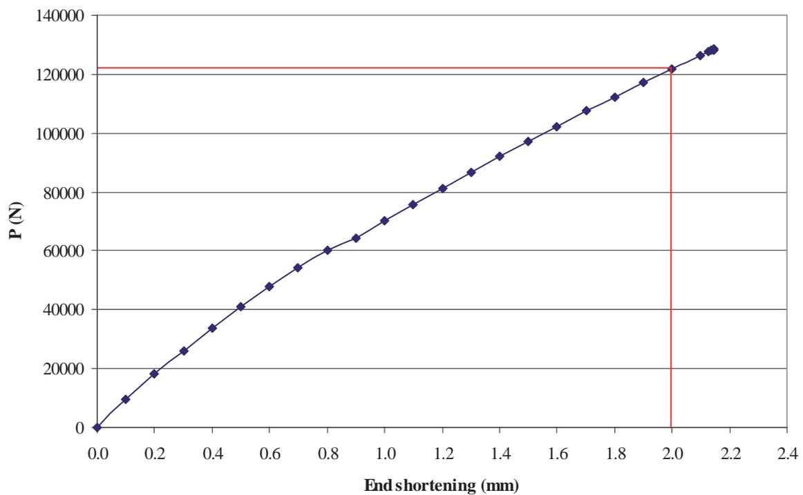
Figure 5: Non linear solution results for the baseline composite panel.
