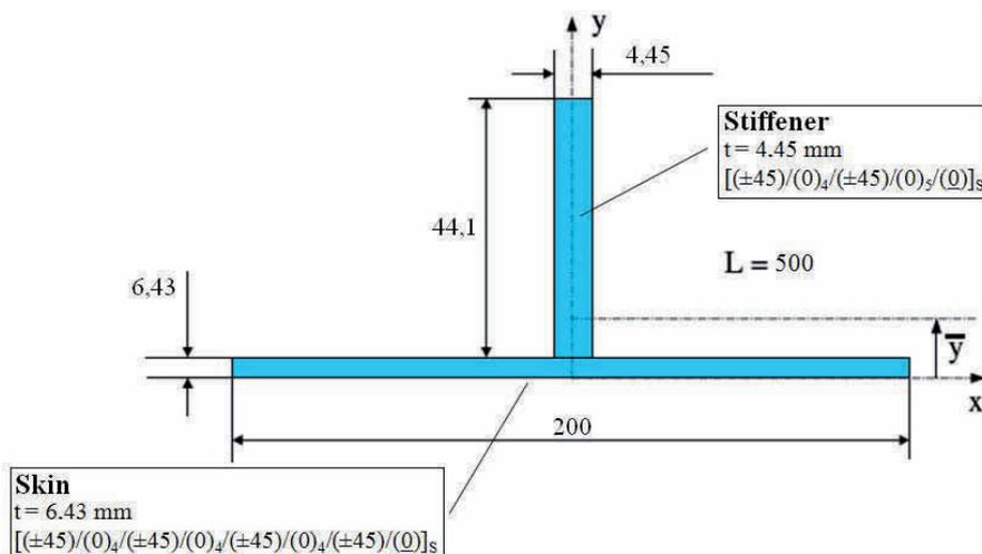
Figure 8: Composite panel with the optimal dimensions of Neto (2006).
