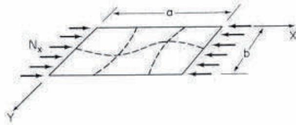
Figure 7: Simple supported plate under axial loads.
