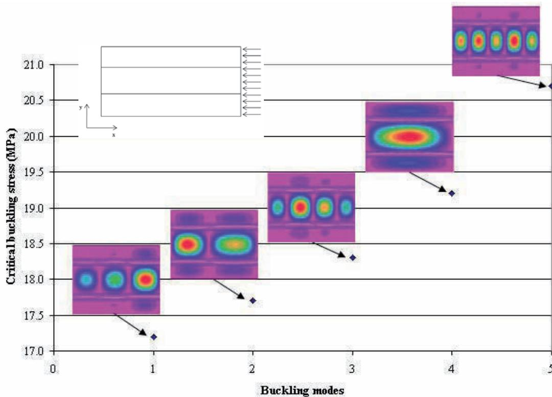
Figure 4: Panel buckling modes (SOL105).
