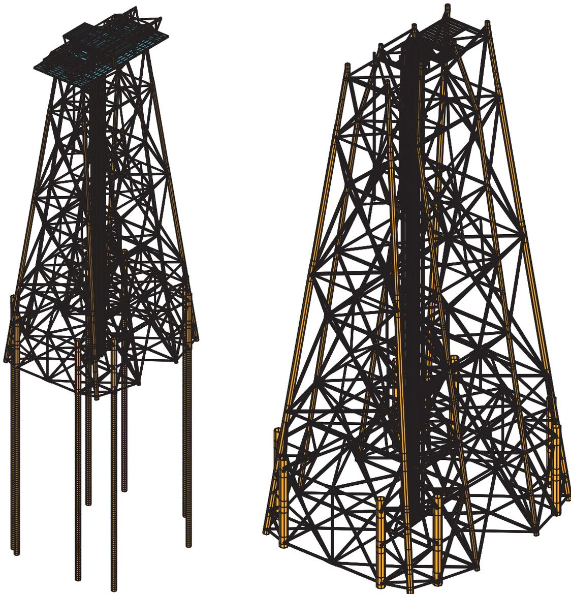
Figure 2: Finite element model: production platform with steel jackets and piles.
