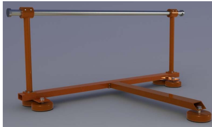
Figure 2: Support apparatus of the tube built for the experimental tests.
