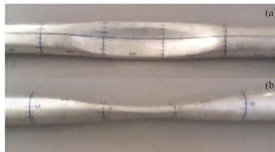
Figure 6: Photos of collapsed tube SE01 after being subjected to 3g explosive from distance of 0.150m (test T11): (a) front view and (b) transverse view.
