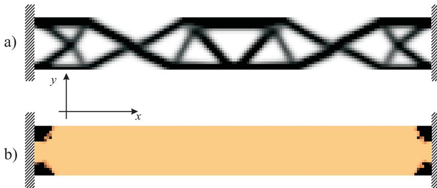
Figure 6: Optimal topologies ( $r_{min}^1 = r_{min}^2$ ). a)  $\rho_1$  b)  $\rho_2$
