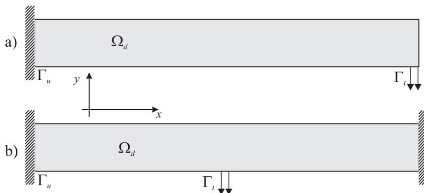
Figure 1: Cantilever beam and beam fixed at both ends
