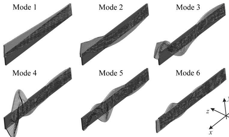
Figure 4: Structure and six modal shapes ( $z$  fixed)
