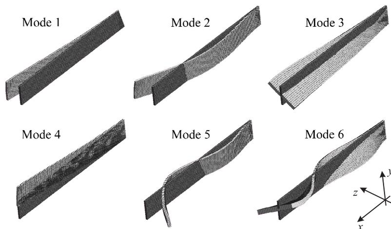
Figure 2: Structure and six modal shapes ( $z$  free).
