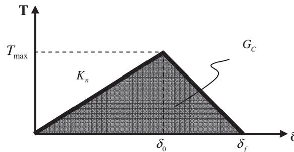
Figure 1 Bi-linear cohesive element traction-separation (T- $\delta$ ) law
