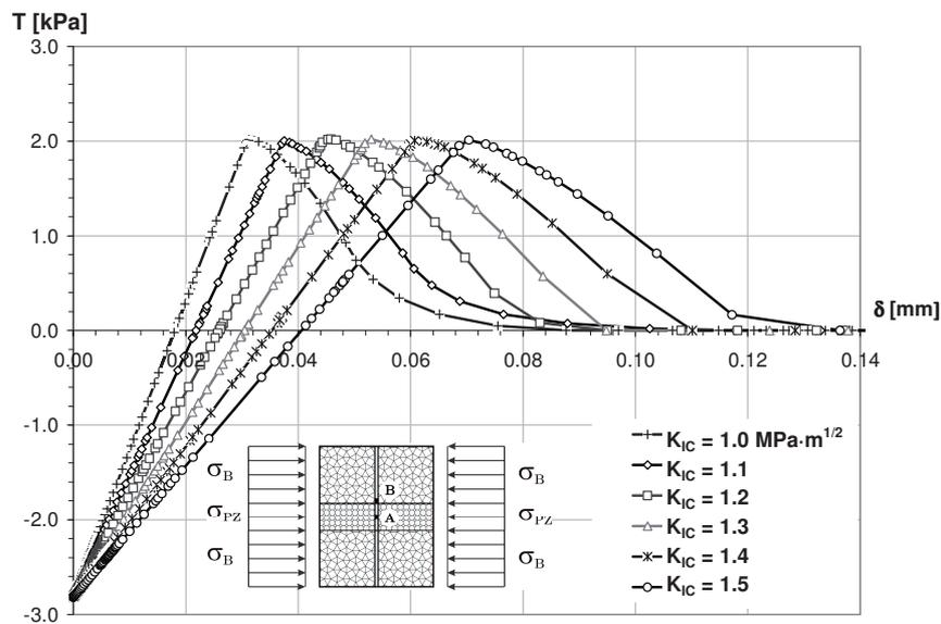
Figure 4 Bi-linear cohesive law at point B in the barrier for different  $K_{IC}$  values
