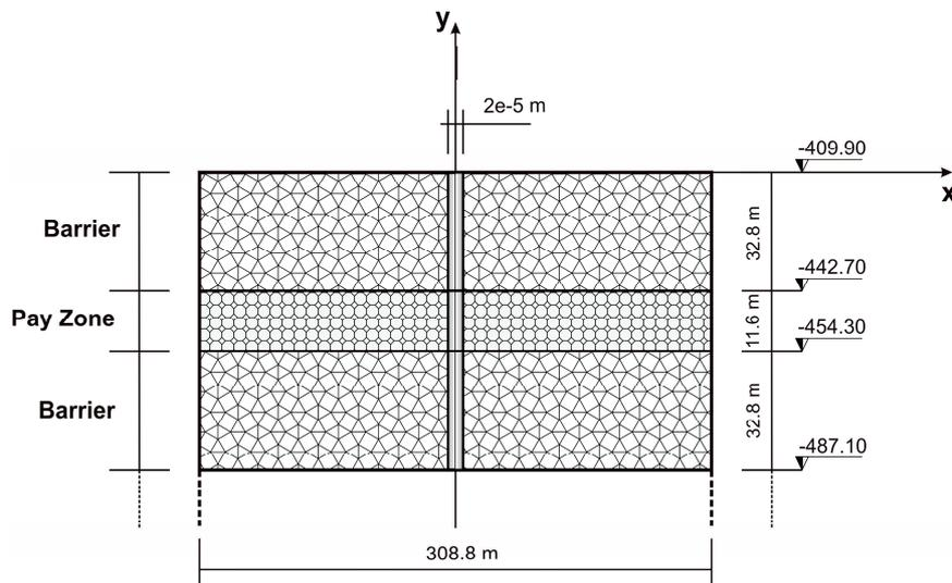
Figure 2 Schematic representation of the formation
