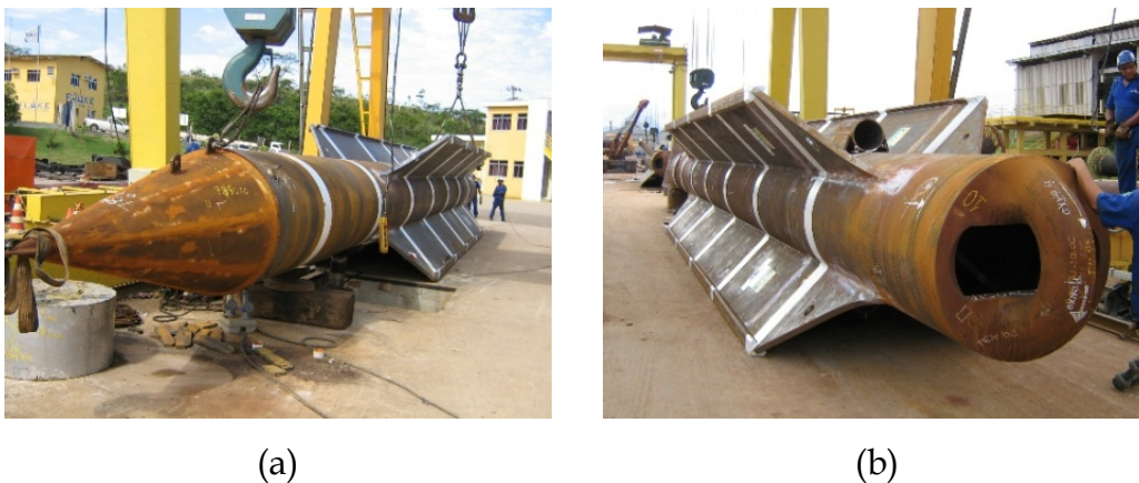
Fig. 1 – Typical torpedo anchor with four flukes: (a) conical tip; (b) top with detail of the padeye.
