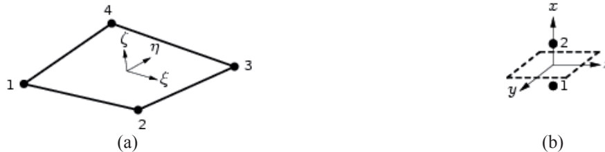
Figure 7: Elements used in numerical modeling (DIANA®).
