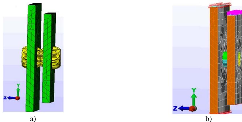
Figure 2. Two configurations of joints. Finite element model. a) bolt modeled as beam; b) perfectly assembled cylinder with distributed load.
