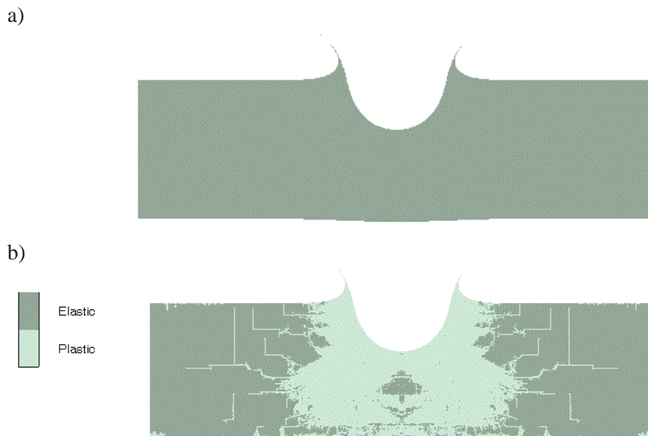
Figure 10: Damaged slab (Numerical simulation 2mm mesh size). Damage failure a) B = 1.6, D_1 = 0.04, D_2 = 1 ; b) B = 0.16, D_1 = 0.004, D_2 = 1
