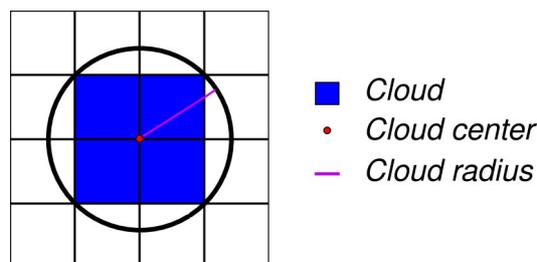
Figure 2: A GFEM mesh: a cloud, its vertex and radius.
