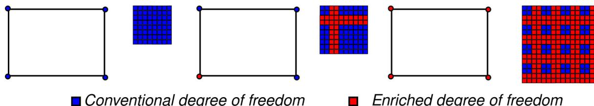
Figure 3: Conventional element matrix and a scheme of the resulting additional lines and columns on its enriched local stiffness matrix.
