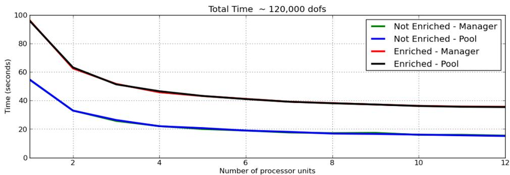
Figure 22: Total solution time for meshes containing around 120,000 degrees of freedom
