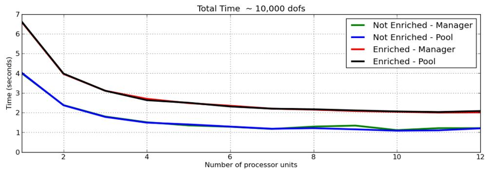
Figure 20: Total solution time for meshes containing around 10,000 degrees of freedom
