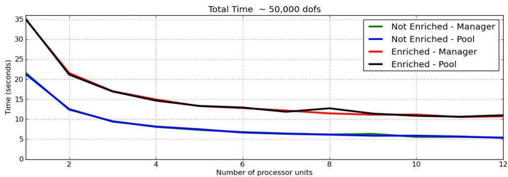
Figure 21: Total solution time for meshes containing around 50,000 degrees of freedom
