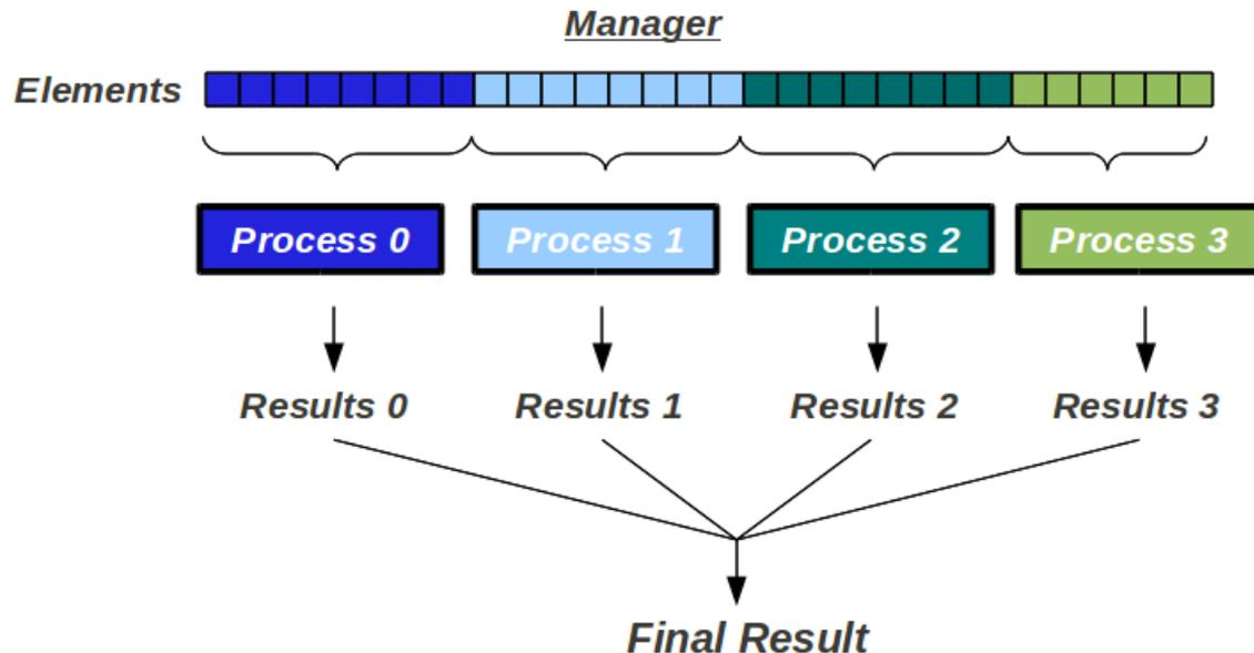
Figure 6: Scheme of the local stiffness matrix and force vector computation using Multiprocessing's Manager.
