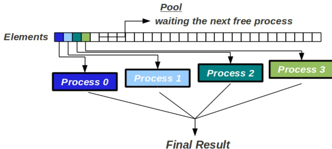
Figure 8: Scheme of the local stiffness matrix and force vector computation using Multiprocessing's Pool.
