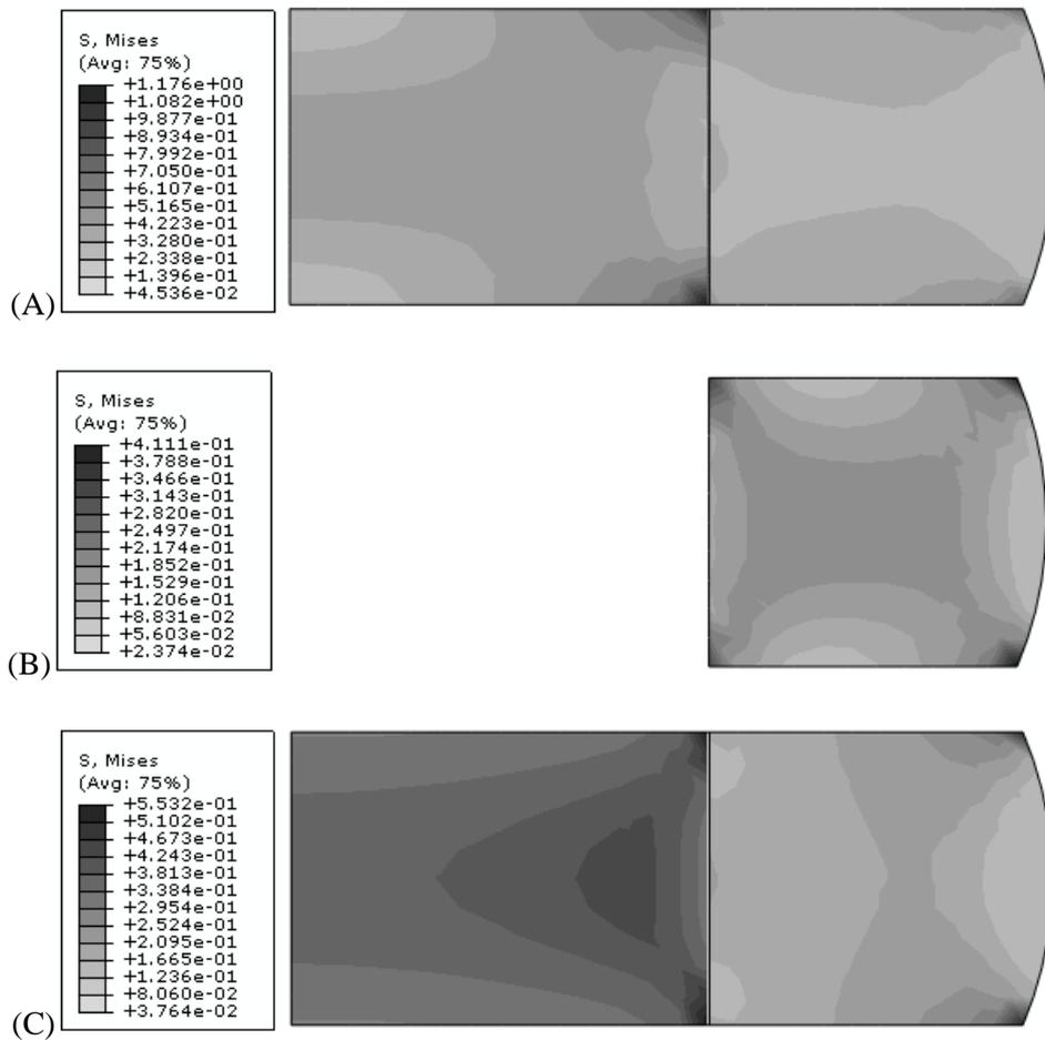
Figure 5: Von Mises stress distributions for (A) intact, (B) denucleated and (C) implanted model. All values in MPa.
