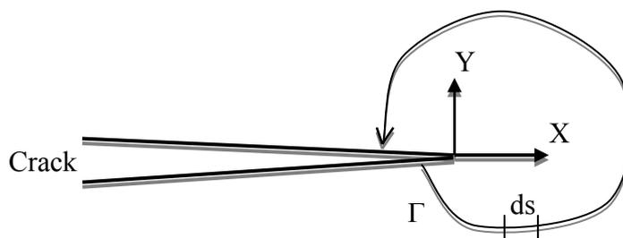
Figure 3: Arbitrary contour  $\Gamma$  surrounding the crack tip
