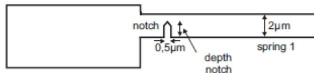
Figure 2: Simulated crack details
