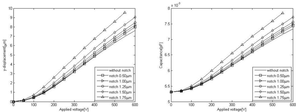
Figure 7: Displacement (left) and Capacity (right) of the comb-drive as a function of the applied voltage
