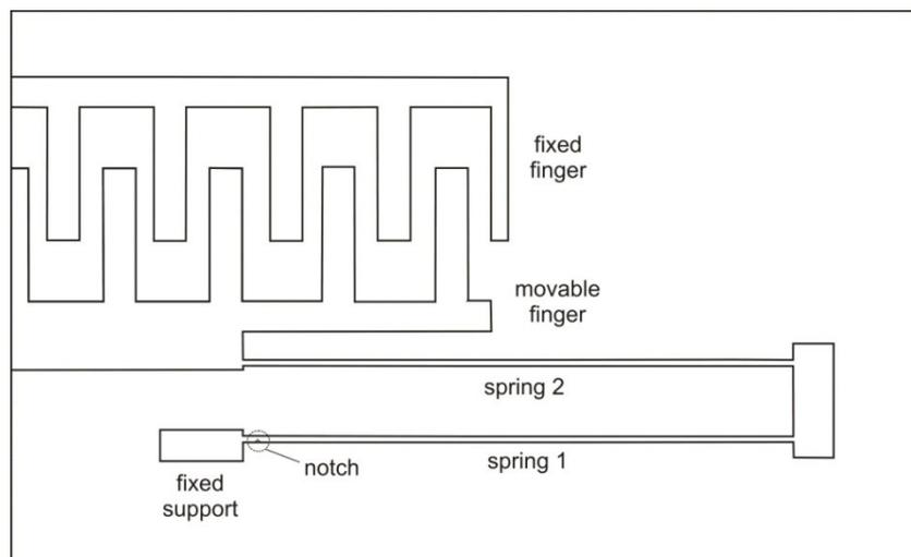
Figure 1: Simulated comb-drive structure
