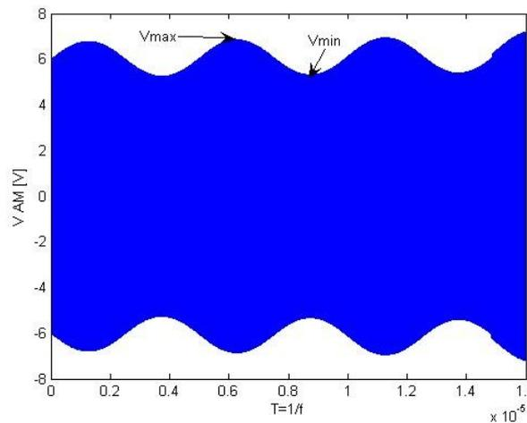
Figure 10: Amplitude modulated signal ( $V_{AM}$ ) obtained at the output of the measurement circuit for a crack depth of 1.5 microns
