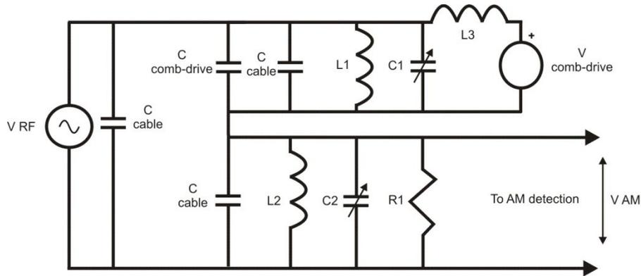
Figure 8: Circuit employed to measure the capacity of the comb-drive
