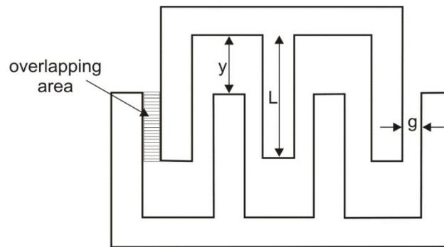
Figure 6: Parameters for measuring capacity in a comb-drive
