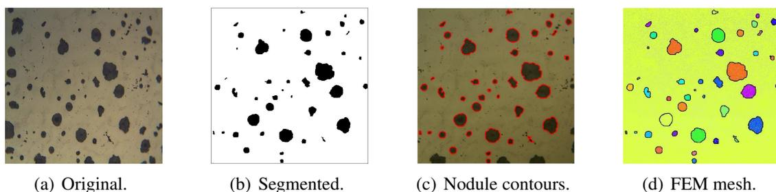
Figure 9: Images corresponding to 14C × 100\_I rectangular sample (see Figure 4(d)).
