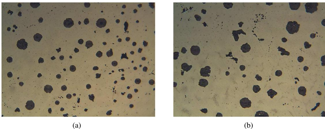
Figure 1: Micrographies of semipearlitic SGI corresponding ar two differents points.
