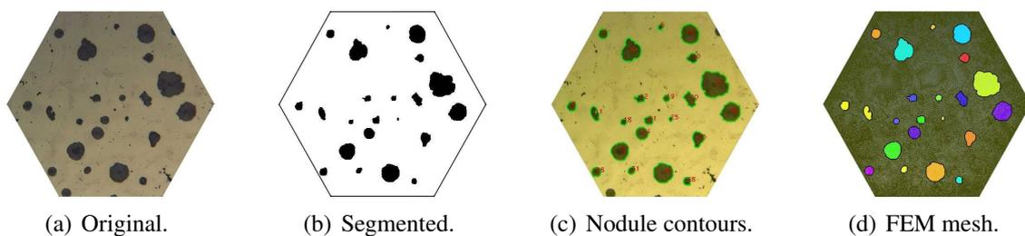
Figure 8: Images corresponding to 14C × 100\_I hexagonal sample (see Figure 4(d)).
