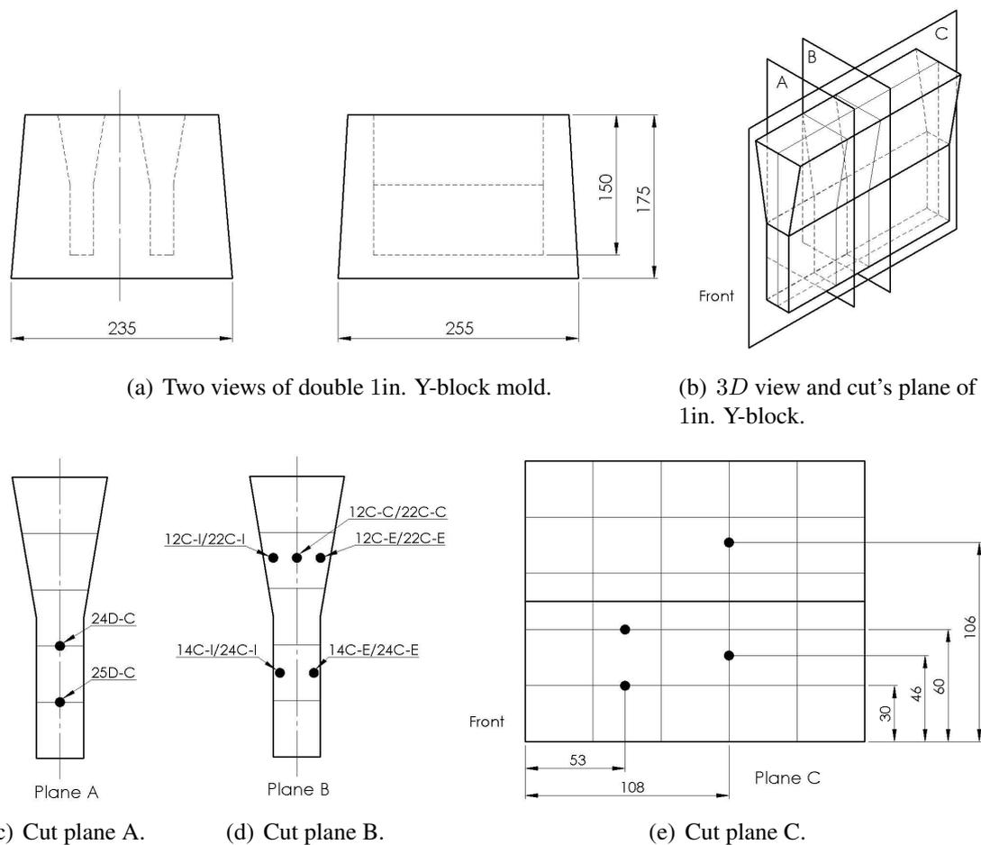
Figure 4: Mold, 1in. Y-block and locations of the samples used for metallurgical study.
