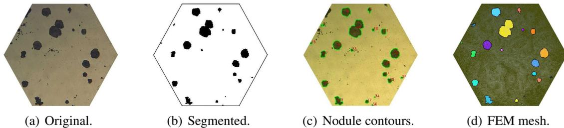
Figure 6: Images corresponding to 14C × 100\_E hexagonal sample (see Figure 4(d)).
