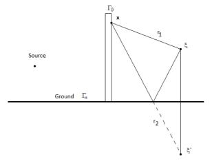
Figure 5 Two dimensional half-space limited by and infinite rigid plane  $\Gamma_H$  and interior boundaries  $\Gamma_0$
