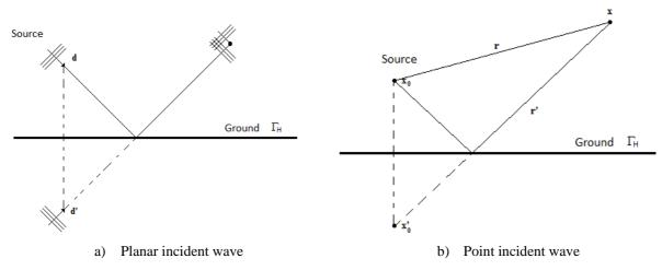
Figure 2 Incident wave reflection of a two-dimensional half-space  $\Omega$  limited by an infinite plane  $\Gamma_{H}$ .
