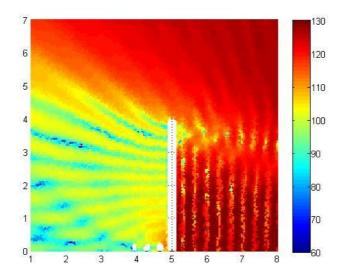
Figure 13 SPL field of the optimized barrier
