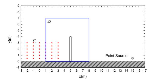
Figure 11 Problem set-up The wavenumber of the incident wave is  $\kappa = 9.9 \text{ m}^{-1}$  and its amplitude is A = 1 Pa. The
