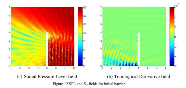
Figure 12 shows the sound pressure level (SPL) and Topological Derivative fields of the barrier. The most negative values of  $D_T$  are on the left hand side of the barrier. Thus, in order to improve this barrier new scatters are placed on the positions with the 20 most negative values of  $D_T$ . The resulting barrier is analyzed to show the improvement, this result is depicted in Figure 13.
