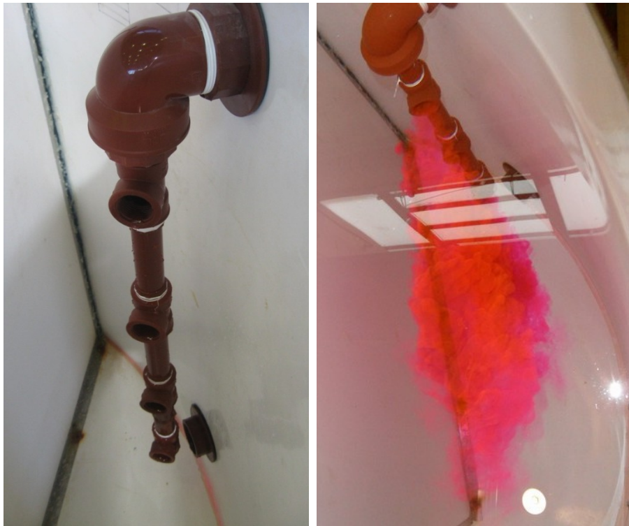
Figure 17: Left: view of the four holes inlet distributor. Right: picture showing the tracer entering to the tank
