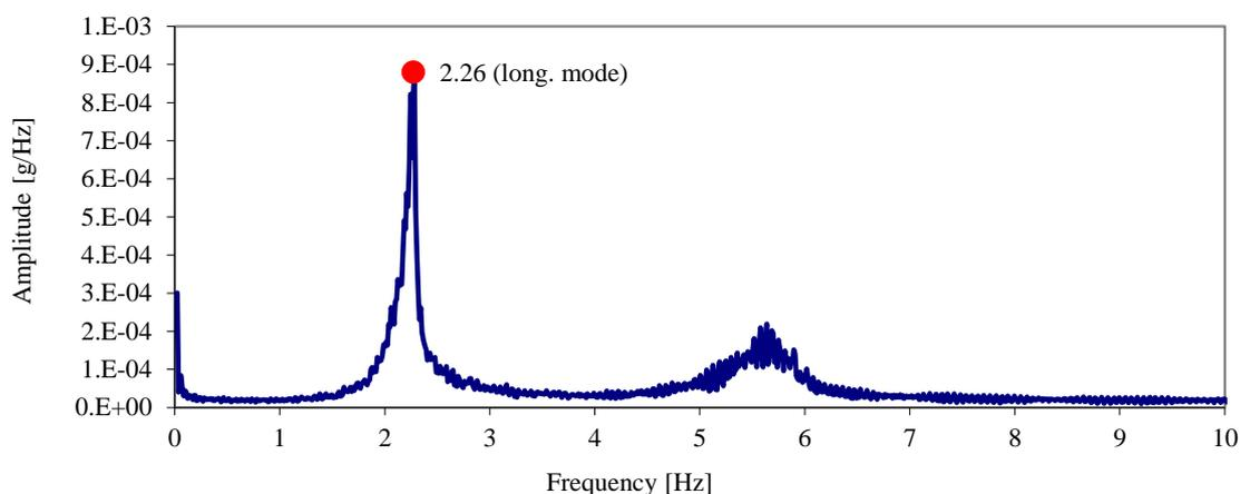
Figure 8: Average Fourier spectrum in the G-FRP frame (25, records with 200 Hz during 1 minute).
