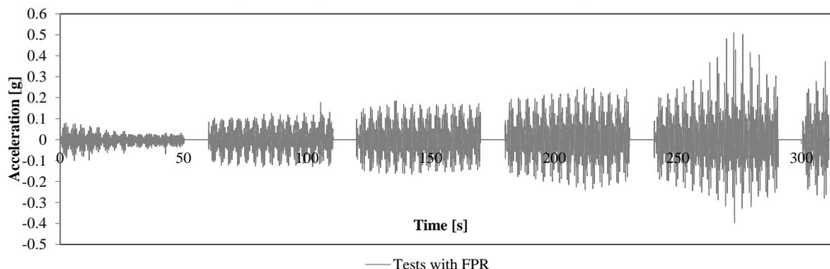
Figure 13: Input acceleration records for the retrofitted frame with G-FRP.
