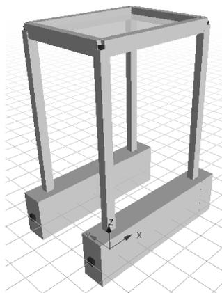
Figure 10: FEM of the frame in SeismoStruct.
