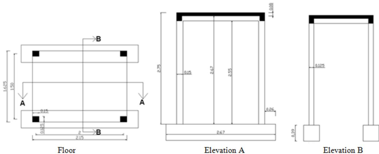
Figure 2: Global dimensions of the prototype.
