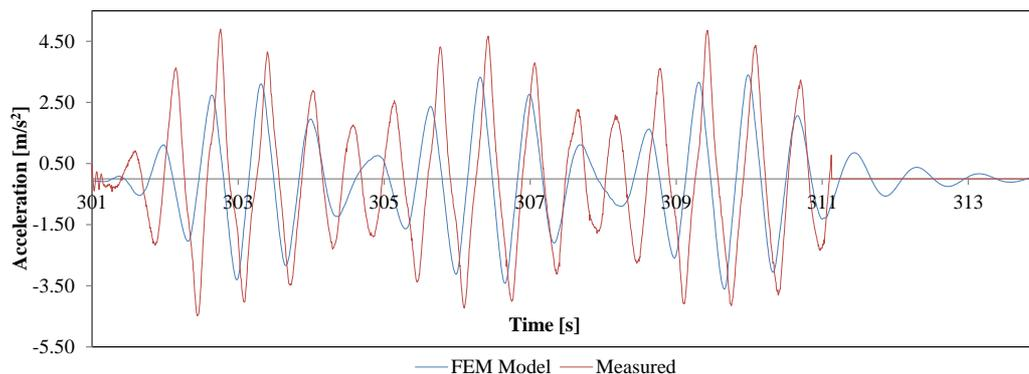
Figure 15: Acceleration time history, numerical vs. experimental measurements for the six tests (Frame with G-FRP).
