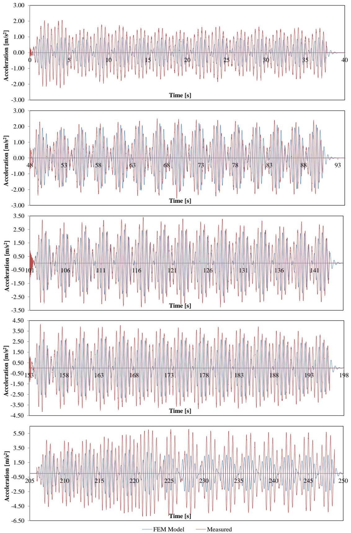
Figure 14: Acceleration time history, numerical vs. experimental measurements for the five tests (Frame without G-FRP).
