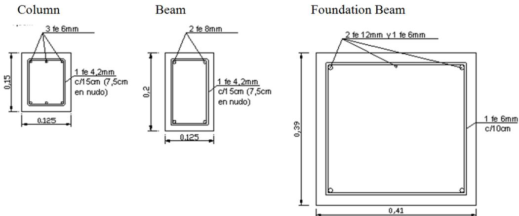
Figure 3: Cross sectional dimensions of the prototype's members.
