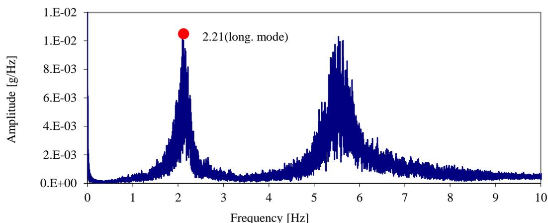
Figure 9: Average Fourier spectrum in the G-FRP frame (9 records, 250 Hz during 20 minute).
