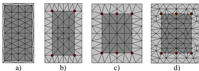
Figure 11: Discretization of Different Elements; a) Foundation Beam (100 fibers), b) Beams (100 fibers), c) Columns (100 fibers) y d) Plastic Hinge zone on Columns (200 fibers).
