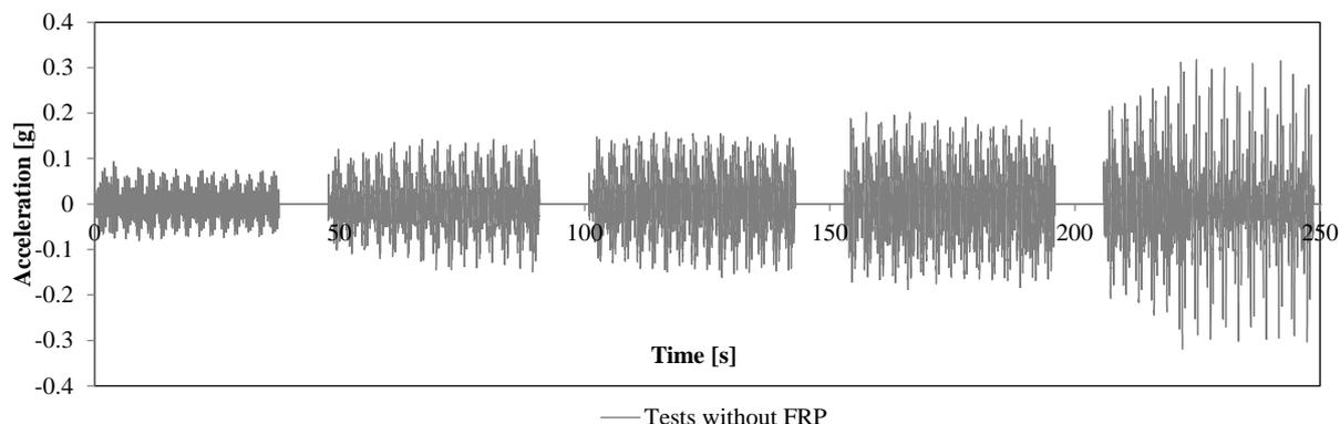
Figure 12: Input acceleration records for the original frame.
