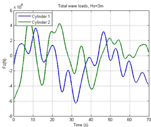
Figure 11: Total wave loads at cylinders
