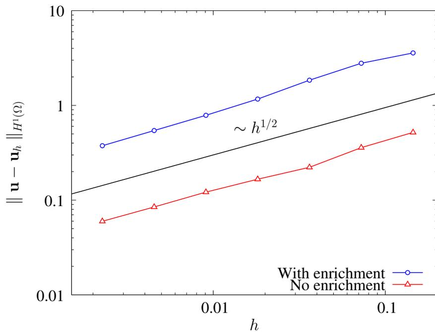
Figure 3:  $H^1(\Omega)$  error norm of the velocity field for the Couette problem using the enrichment (circles) and without the enrichment (triangles).
