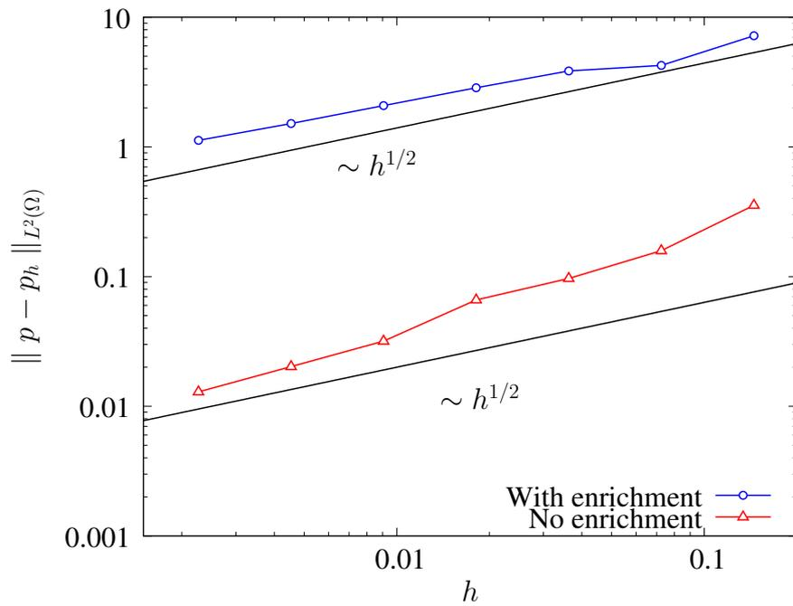
Figure 2:  $L^2(\Omega)$  error norm of the pressure field for the Couette problem using the enrichment (circles) and without the enrichment (triangles).
