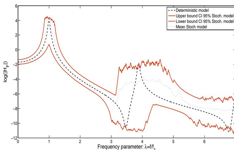
Figure 6: FRF for a nano-beam with high dispersion in non-local parameter and material properties.
