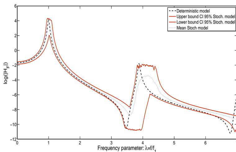
Figure 4: FRF for a nano-beam with low dispersion in non-local parameter and material properties.
