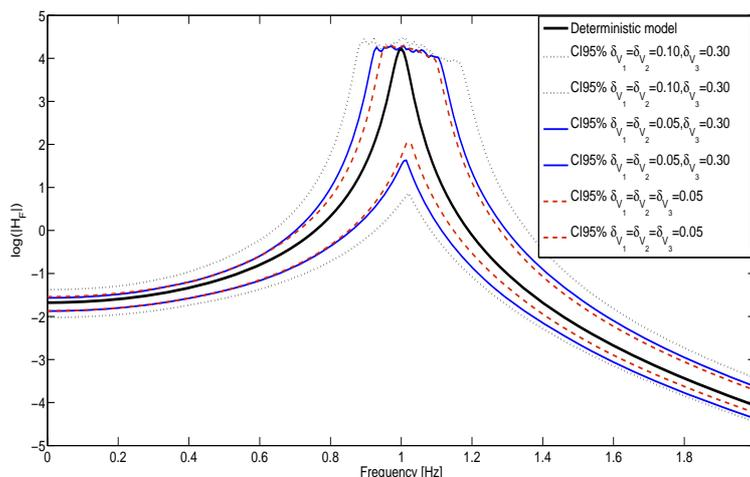
Figure 7: Comparison of the uncertainty propagation near the first mode.
