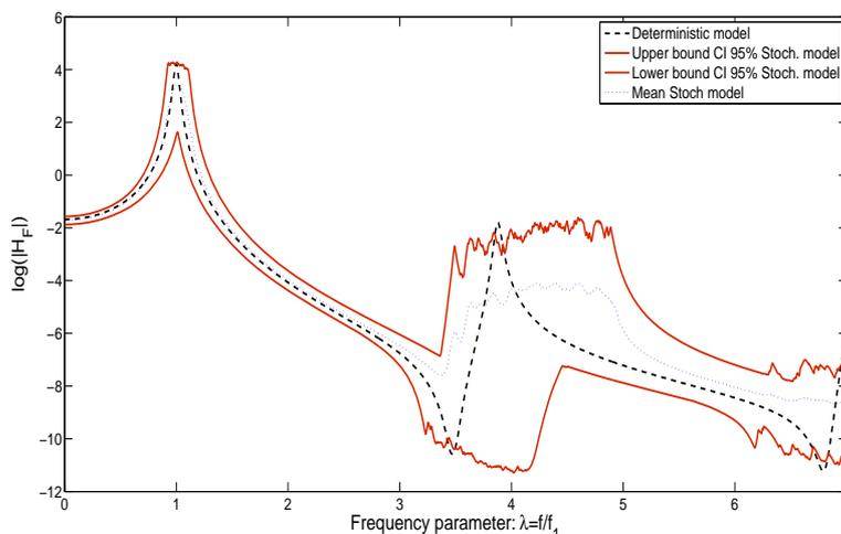
Figure 5: FRF for a nano-beam with high dispersion in non-local parameter and low dispersion in material properties
