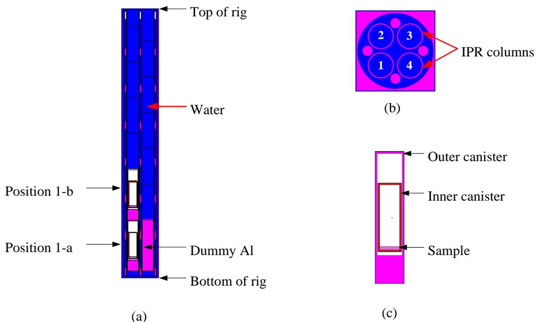
Figure 5: MCNP model of IPR and samples
