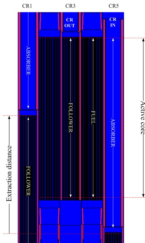
Figure 3: Illustration of possible axial control rod positioning
