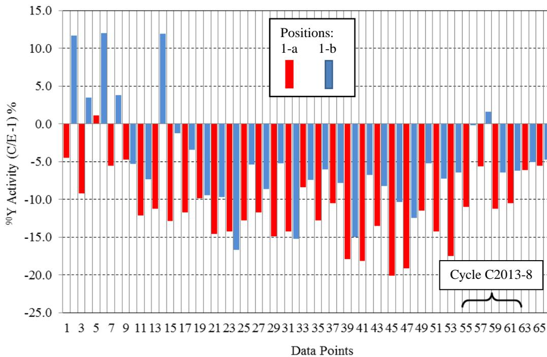
Figure 11:  $^{90}\text{Y}$  activity comparison between calculation and experiment  $[(C/E - 1) \%$  ]
