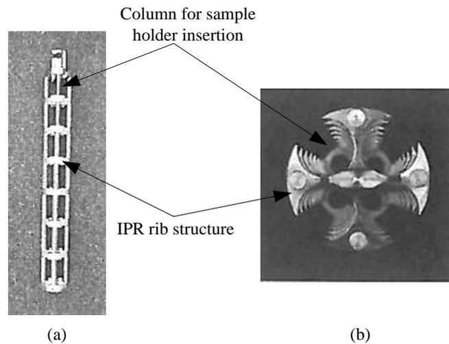
Figure 4: (a) Side view of IPR, (b) Top view of IPR
