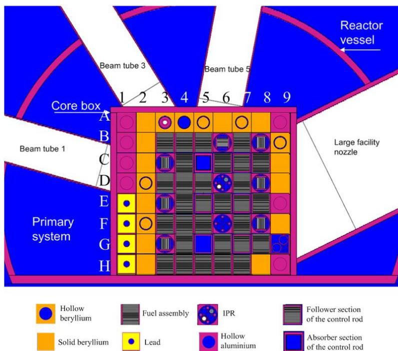
Figure 1: XY view of the core and beam tubes
