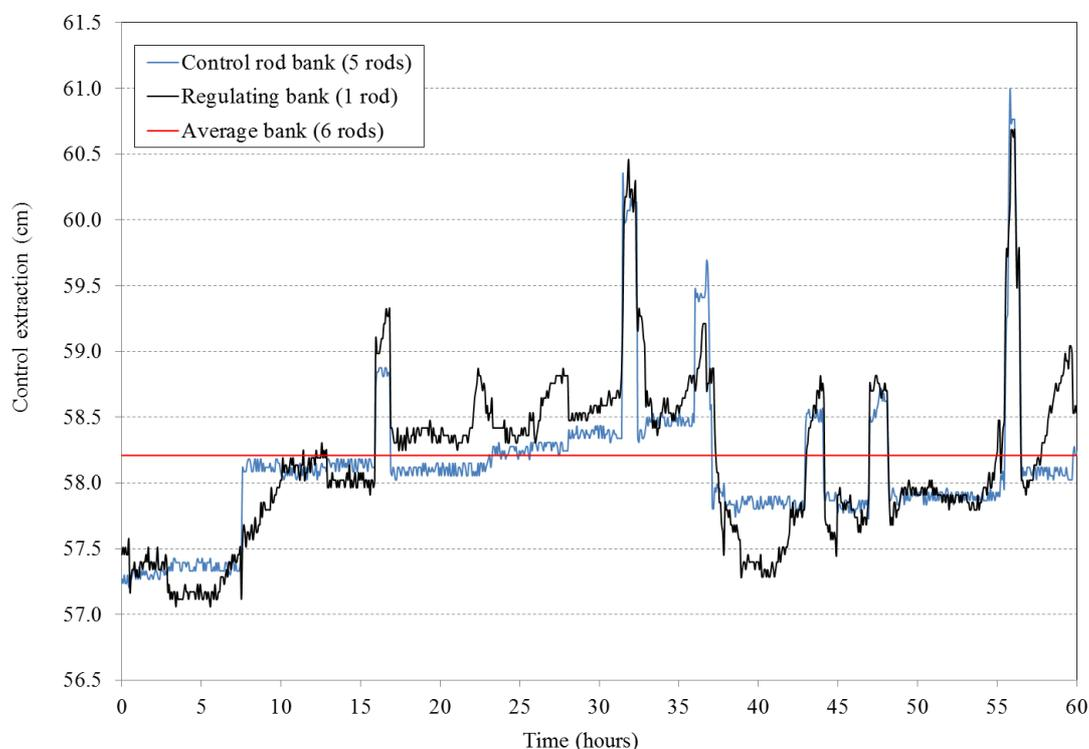
Figure 8: Example of control rod bank movement during irradiation
