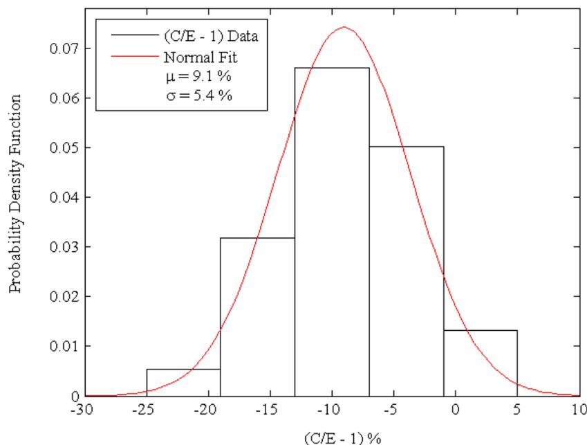
Figure 12: Gaussian fit to  $^{90}\text{Y}$  activity difference in position 1-a
