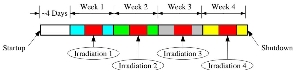
Figure 9: Schematic representation of typical sample irradiation during the depletion cycle
