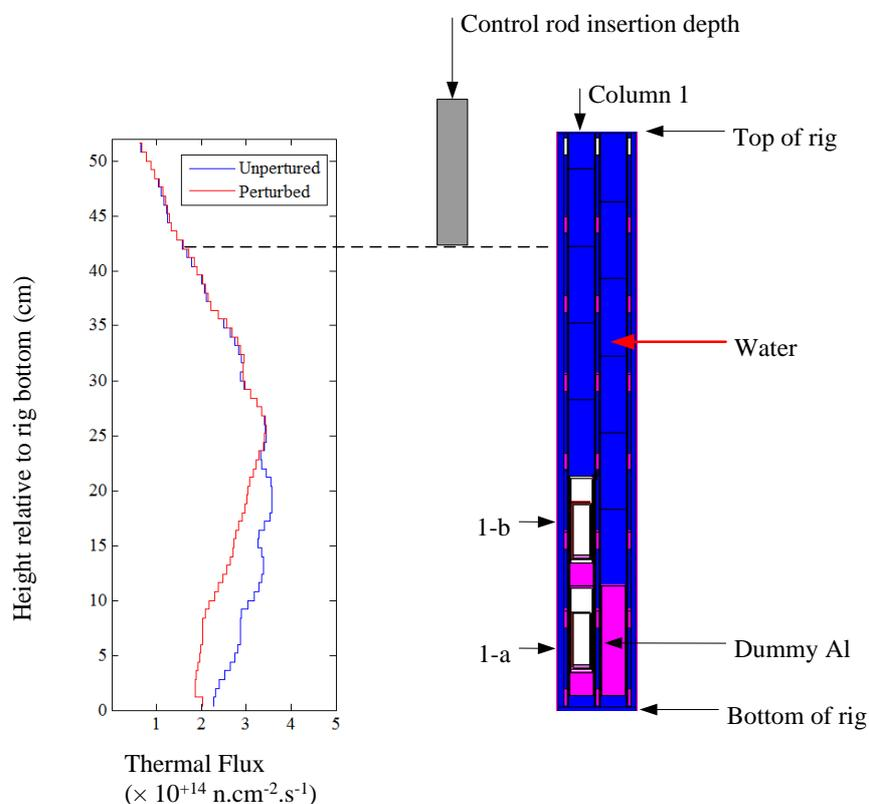
Figure 10: Example of thermal flux suppression in column 1
